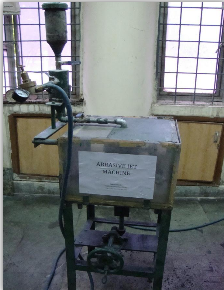
Fig. 8 Abrasive Jet Machine (improved), Metal forming lab Department Of Mechanical Engg. DTU
