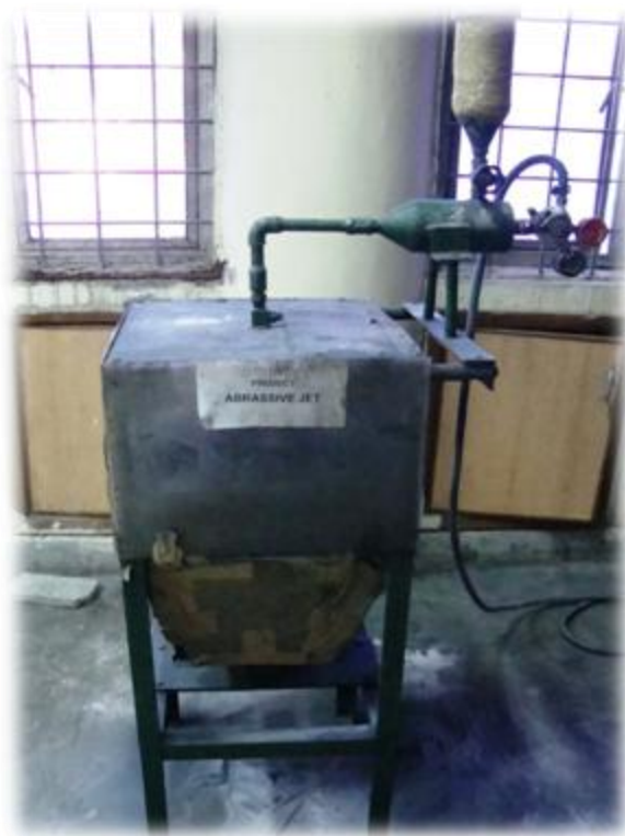
Fig.6 Previous Set-up of Abrasive Jet Machine Metal forming lab Department Of Mechanical Engg. DTU
