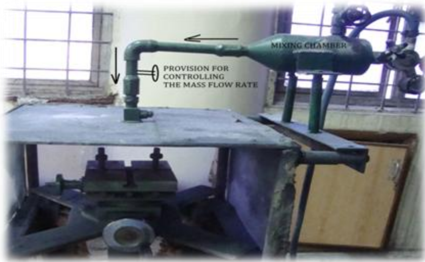
Fig.7 Limitations of Previous Set-up of Abrasive Jet Machine.
