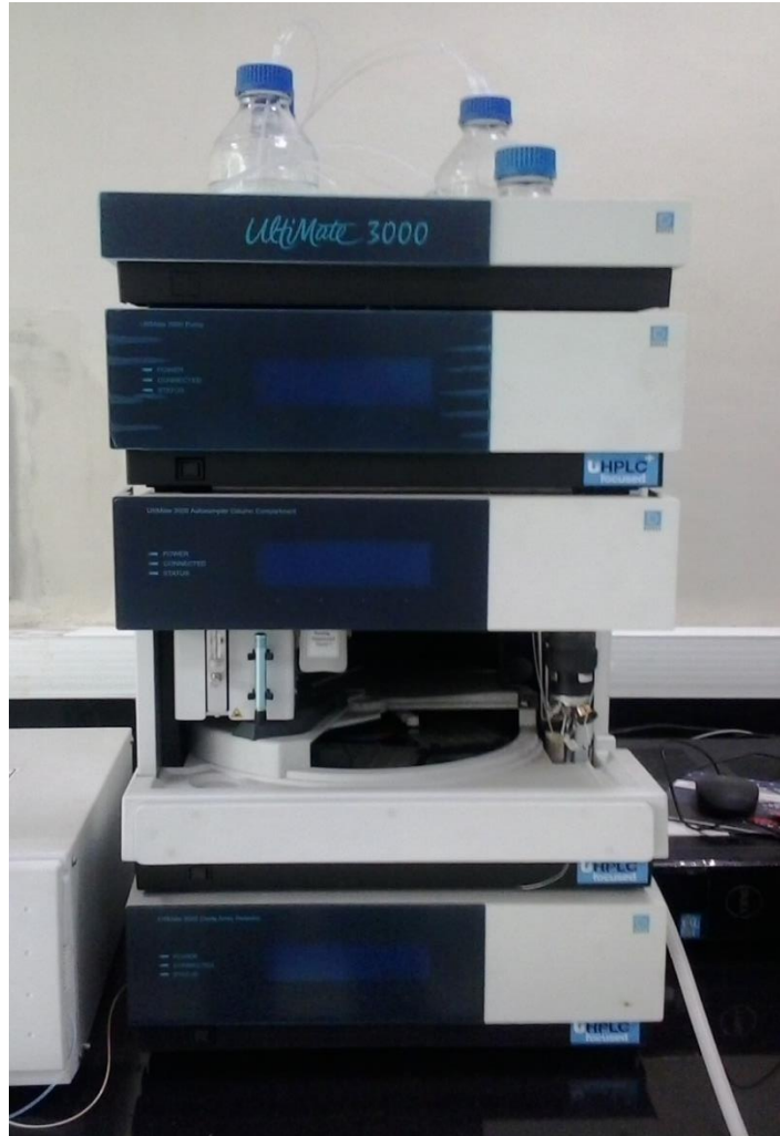
Fig 3.5: Dionex HPLC equipment
