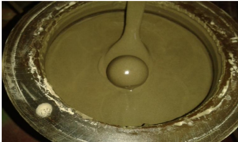
Figure 3.9 Picture showing wet grinding of cement in ball mill machine chamber.
