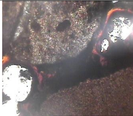
Figure 3.17 d: Another View of photomicrograph of fine sized dry grinded cement and fine aggregate mix, showing dense cement phase and micro-pores with good contact between cement paste and aggregate grains (magnification 60X under polarized light).
