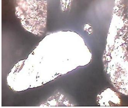
Figure 3.18 a: Photomicrograph of fine sized wet grinded cement and fine aggregate mix, showing dense cement phase and good contact between cement paste and aggregate grains (magnification 60X under non polarized light).
