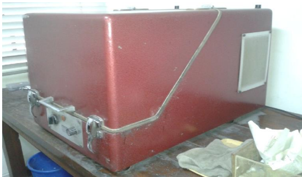
Figure 3.7 Ball mill machine used for the conversion.
