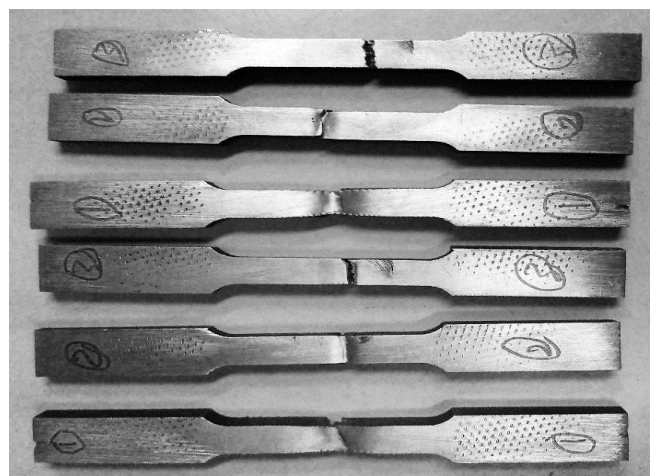
Figure 7. Samples Showing the Failure Regions.
