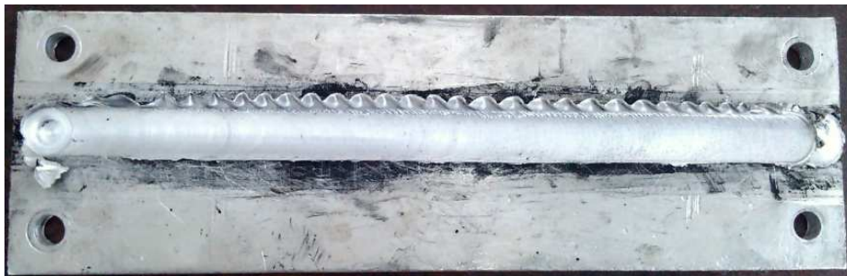
Figure 13. Flash observed on the retreating side of the joint.
