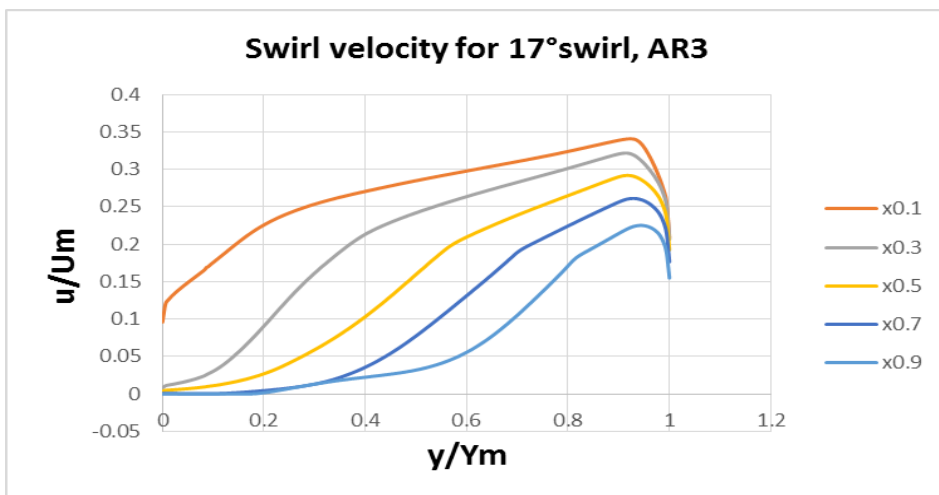
Fig.99 AR=3, Casing wall angle=8°, Velocity=60m/s (17°S)
