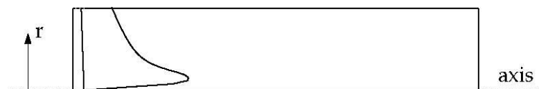
Typical Radial Distribution of \omega in a Free Vortex
