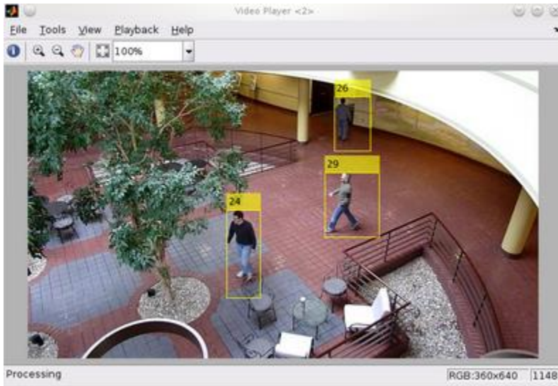
Fig. Tracking of multiple objects using Kalman filter
