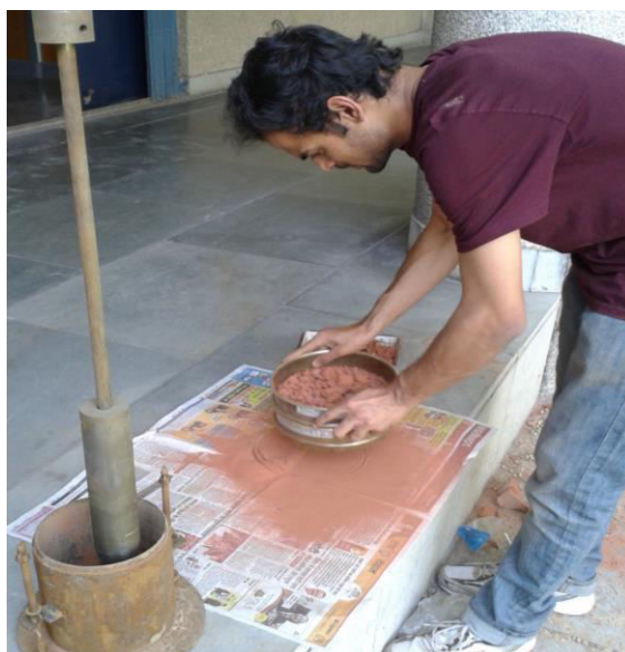
Figure 3.2: Converting brick into smaller particles and then passing through sieve (150-300 microns)
