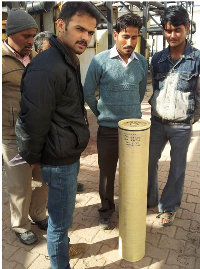
Figure 2.8: A filter from a large size De-fluoridation and De-salination plant at Nagaur (Rajasthan)
