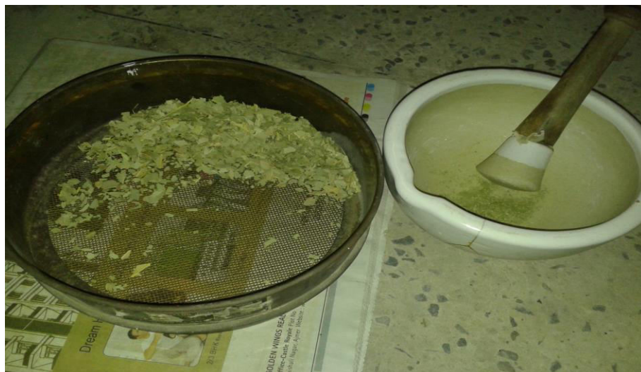
Figure 3.1: Eucalyptus leaves being converted to smaller particles to facilitate adsorption.
