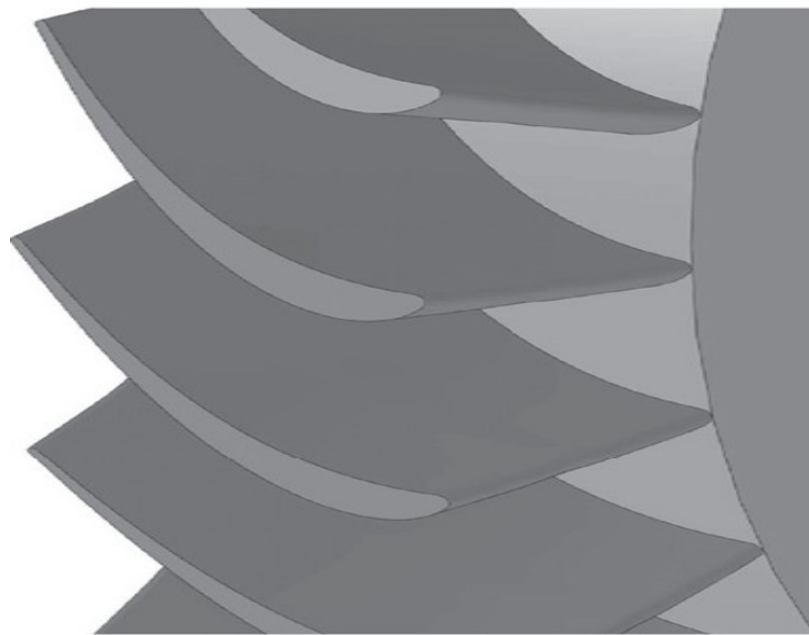
Fig 1.6: 3D turbine blade stacked along the center of gravity (CG)
