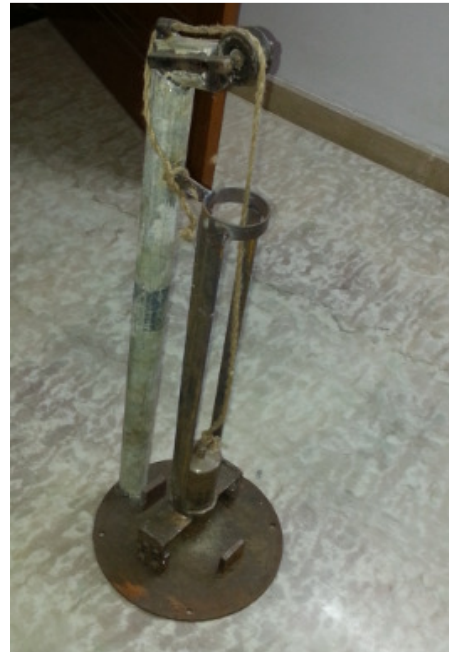
Figure 14: Impact testing machine fabricated in accordance to specifications given in ACI-544.
