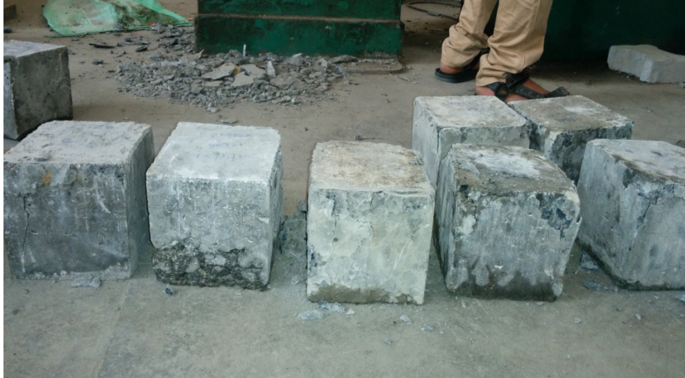
Figure 11: Failure pattern under compressive strength test- Rubber concrete
