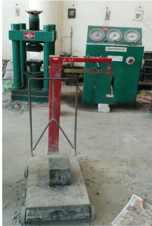
Figure 7: Self weight testing for concrete cube
