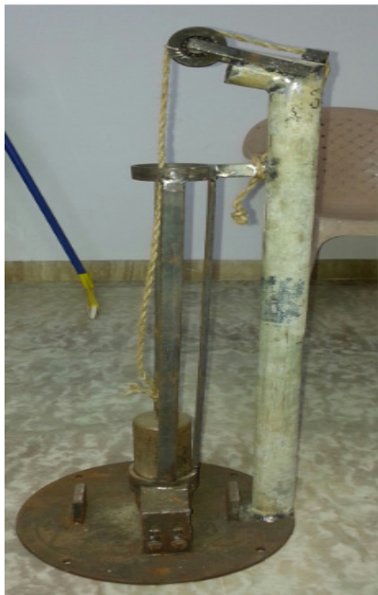
Figure 14: Impact testing machine fabricated in accordance to specifications given in ACI-544.
