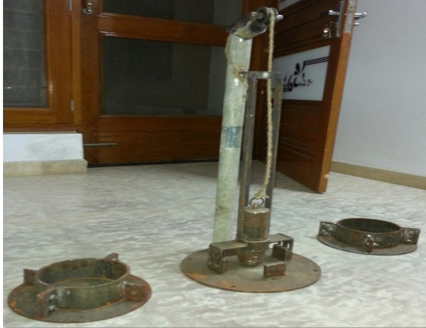
Figure 15: Impact testing machine and molds fabricated according to the specifications given in ACI-544 report
