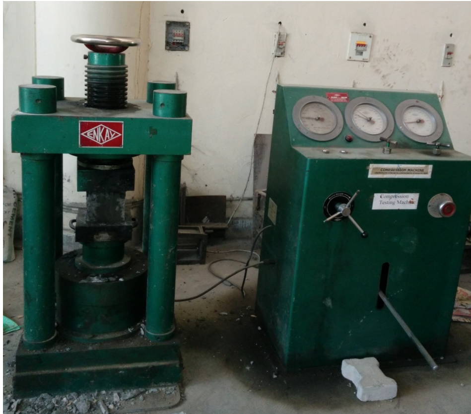
Figure 9: Compressive strength testing machine
