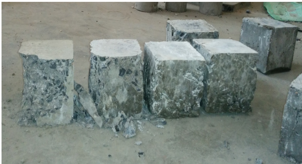
Figure 12: Failure pattern under compressive strength test- Control concrete
