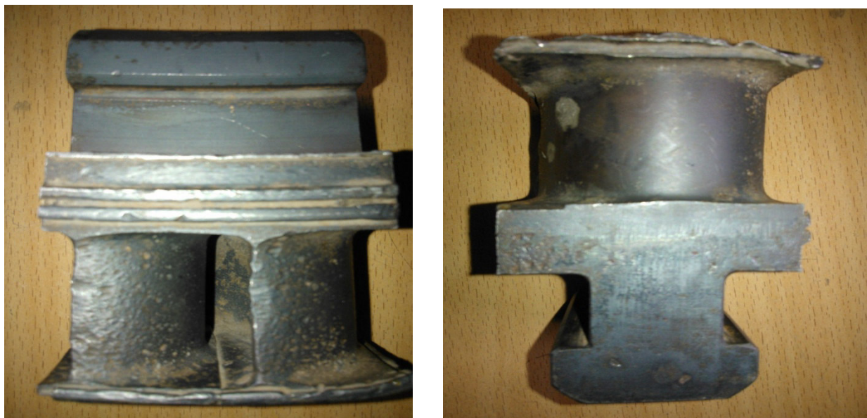
Figure 4.2: leading edge and the suction surface of a turbine blade effected by the particles
