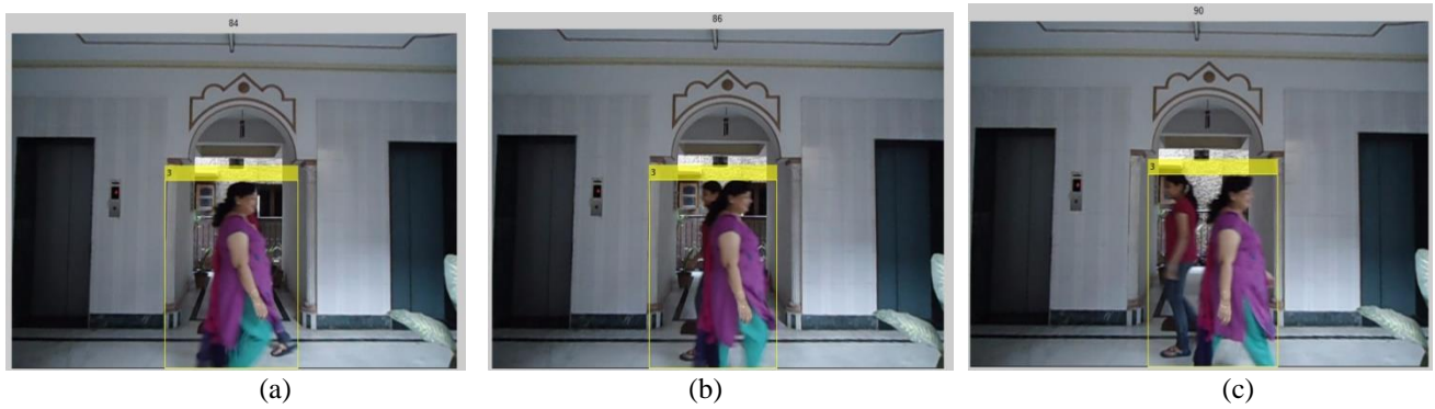
Figure 8. Tracking results of a general Particle Filter. (a), (b) shows tracking during full occlusion between target 1& 2 only one combined target is detected, (c) shows even during partial occlusion only one target is detected instead of two.
