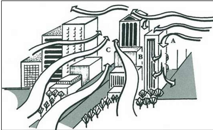
Figure 7.11 - Airflow around different structures such as tall and short buildings, streets
