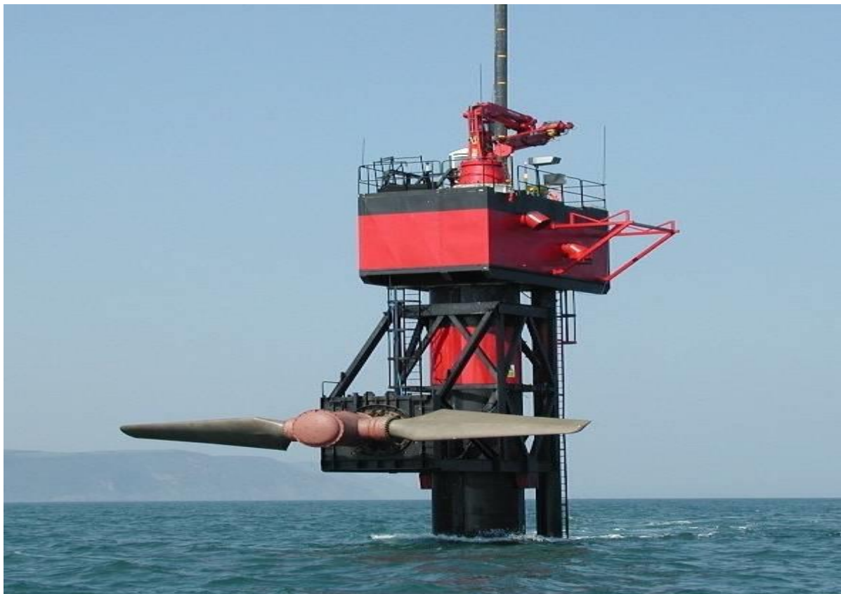
Fig. 2.5 SeaFlow rotor (Courtesy of Marine Current Turbines (MCT) Ltd.).
