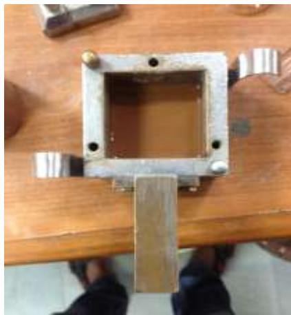
Fig. 4.10 Placement of bentonite layer on lower half of compacted soil
