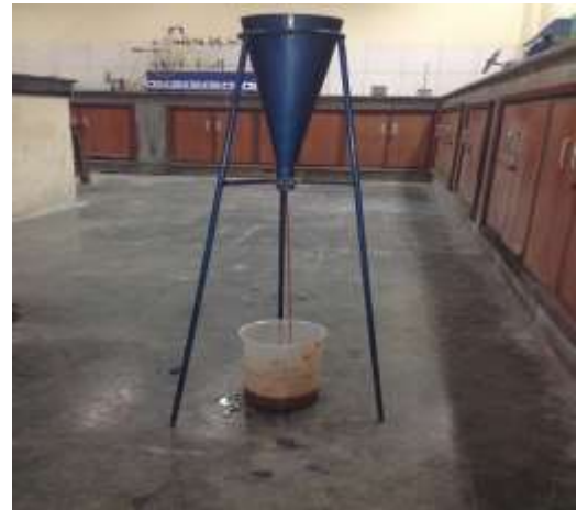
Fig. 3.3 Marsh funnel apparatus
