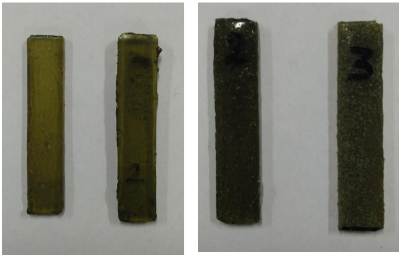
Figure 2.12: Photographs of samples a) neat Vinyl ester b) Microspheres reinforced vinyl ester
