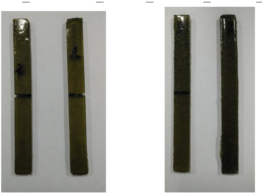
Figure 2.10: Photographs of samples a) neat Vinyl ester b) Microspheres filled vinyl ester
