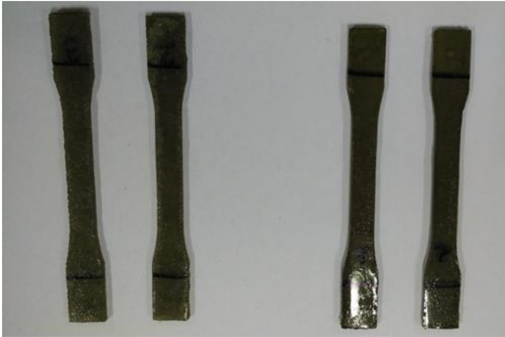
Figure 2.9: Photographs of samples a) Microspheres reinforced vinyl ester b) neat Vinyl ester
