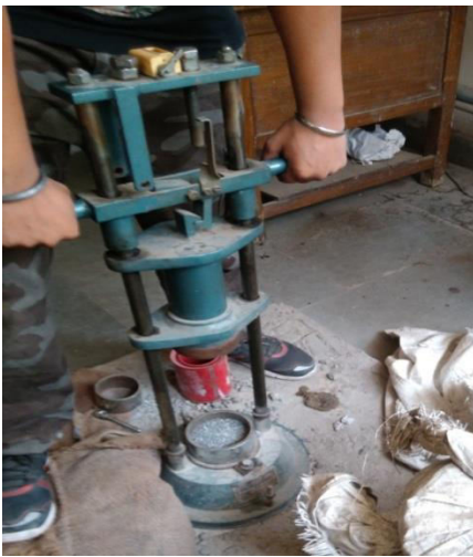
Fig. 3.5 Impact test for crushing value of stone aggregate
