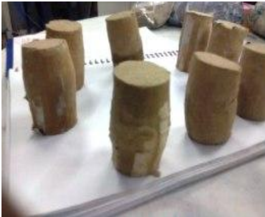
Photograph 4: Bulged sample after shearing
