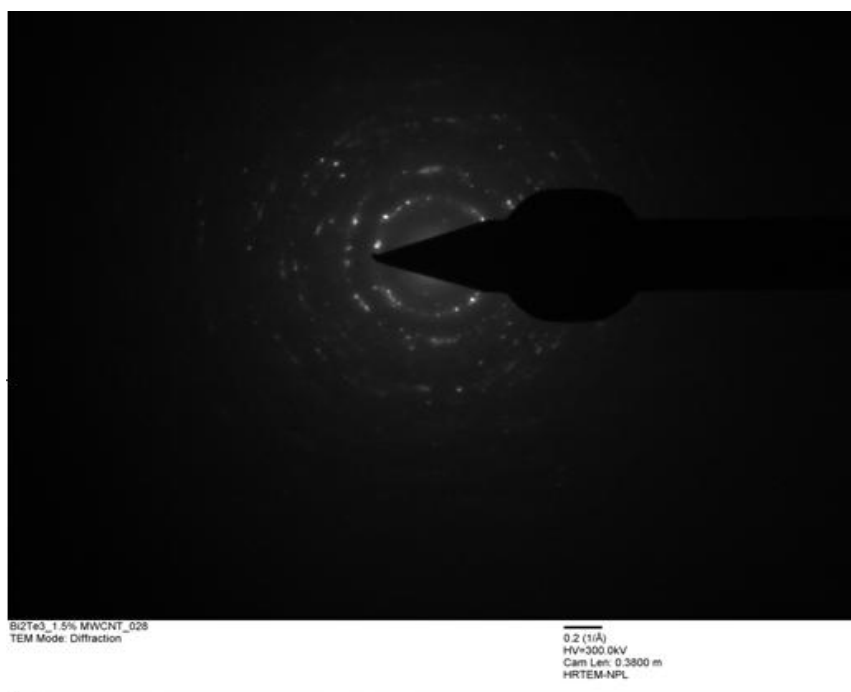
Figure 5.5 SAEDP of 1.5% by weight CNT reinforced \text{Bi}_2\text{Te}_3 .
