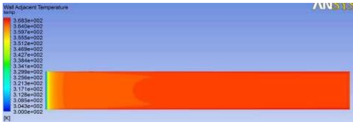
Fig. 5.88 Contours of wall adjacent temperature, Re 3200, without vortex generators
