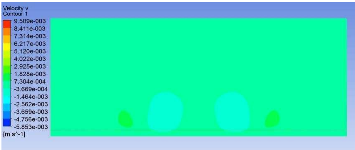
5.102 Contour of v velocity, Re 2400, \beta = 45^\circ (yz plane, x=45 cm)
