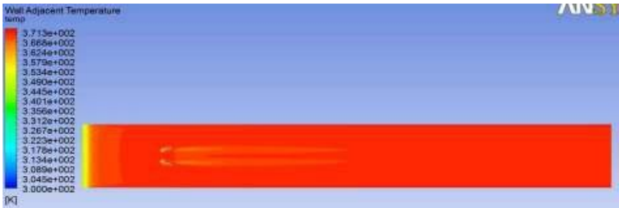
Fig. 5.36 Contours of wall adjacent temperature, Re 2400, \beta = 15^\circ
