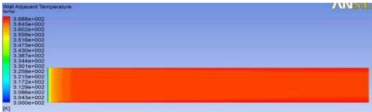
Fig. 5.35 Contours of wall adjacent temperature, Re 2400, without vortex generators
