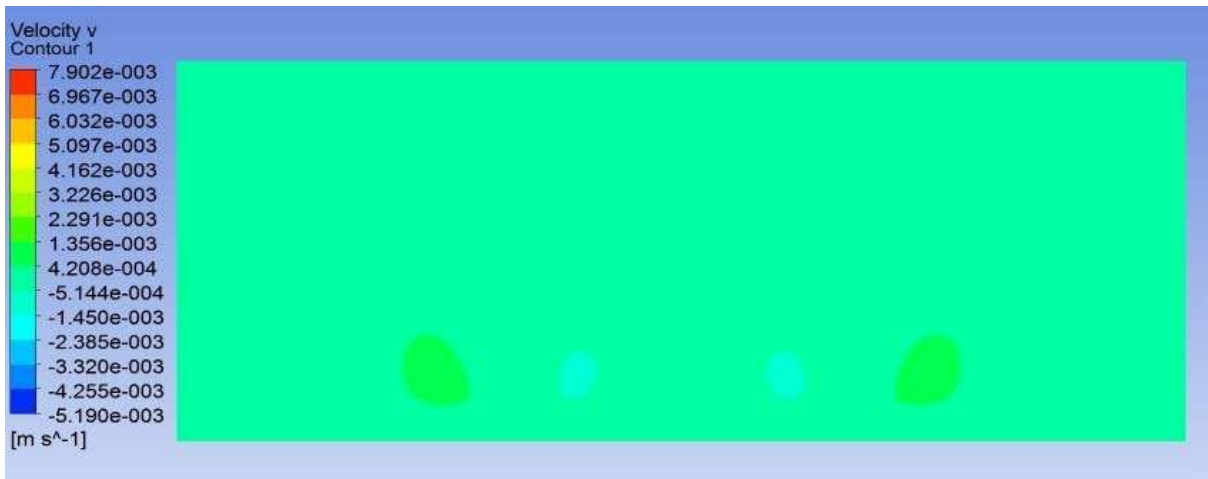
Fig.5.54 Contours of v velocity, Re 2400, \beta = 30^\circ (yz plane, x=60 cm)
