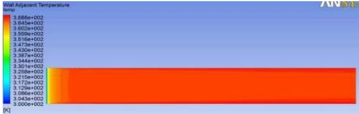
Fig. 5.86 Contours of wall adjacent temperature, Re 2400, without vortex generators
