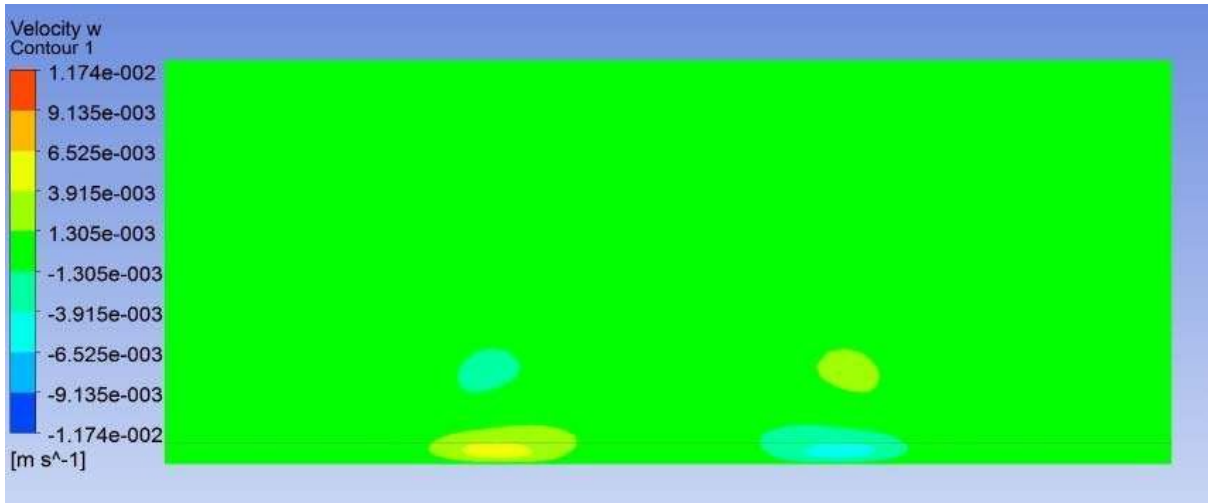
5.106 Contours of w velocity, Re 2400 , \beta = 45^\circ (yz plane, x=40 cm)
