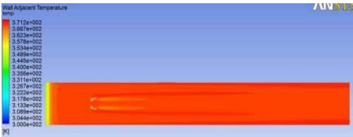
Fig. 5.38 Contours of wall adjacent temperature, Re 3200, \beta = 15^\circ
