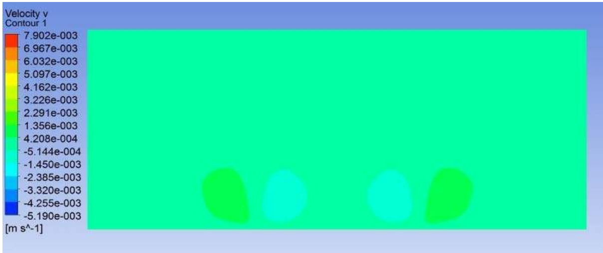
Fig. 5.53 Contours of v velocity, Re 2400, \beta = 30^\circ (yz plane, x=45 cm)
