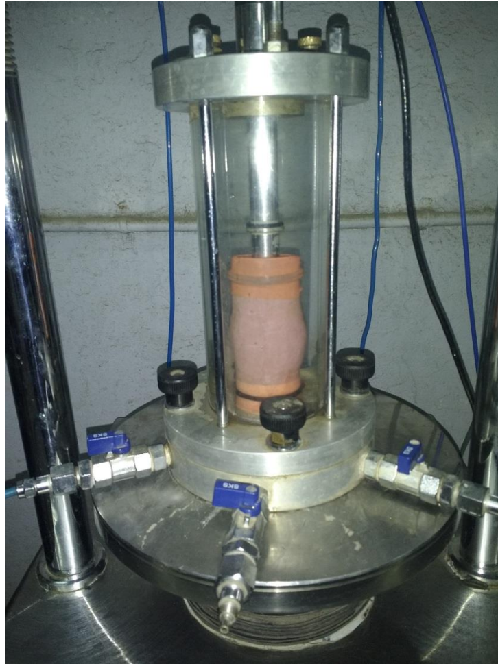
Figur6.5 Failure of Triaxial sample showing bulging
