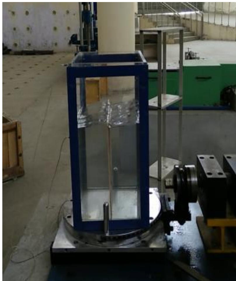
Figure 5.6: Surface profile at 50% fill at frequency 2.8Hz with baffle height 0.3m
