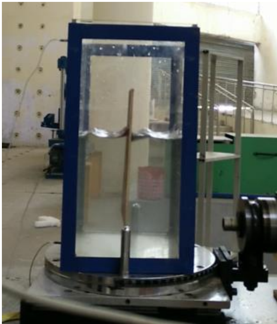
Figure 5.12: Surface profile at 50% fill at frequency 4.4Hz with baffle height 0.4m
