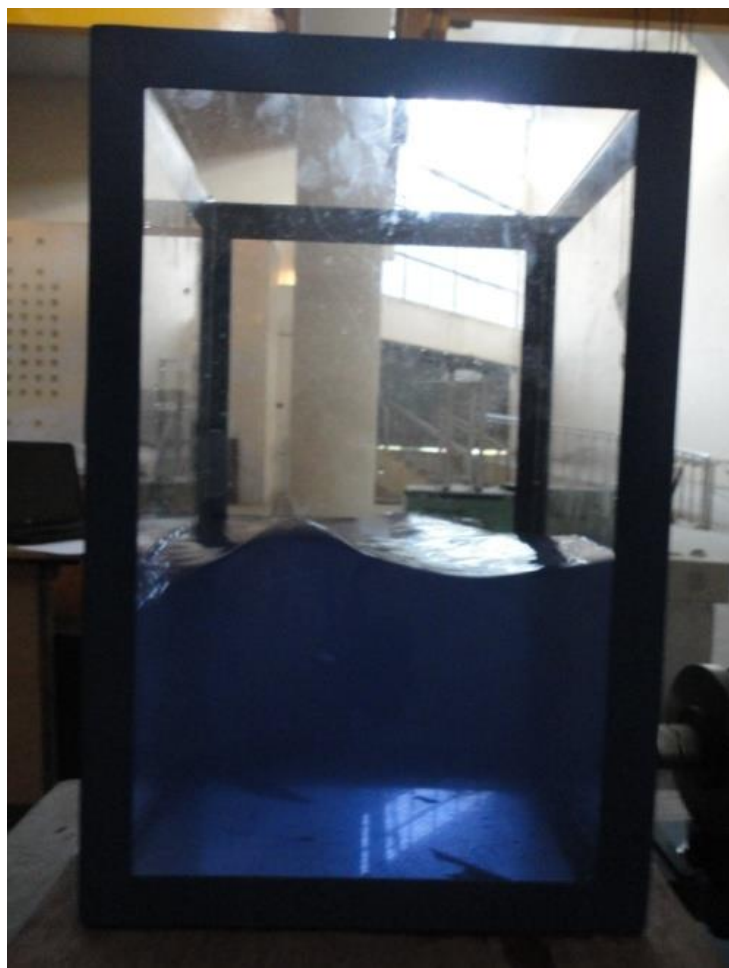
Figure 5.3: Surface profile at second mode ( f_n= 2.8\text{Hz} )
