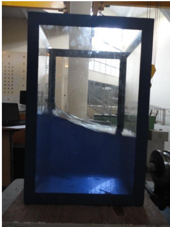
Figure 5.2: Surface profile at first mode ( f_n= 1.6\text{Hz} )
