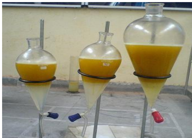
Figure 3.4 - Washing process of biodiesel
