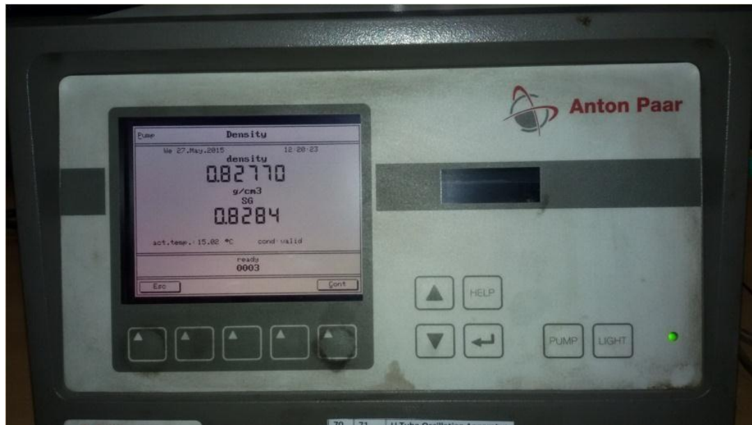
Figure 5.5 - Density Meter showing density and specific gravity for blend B-20
