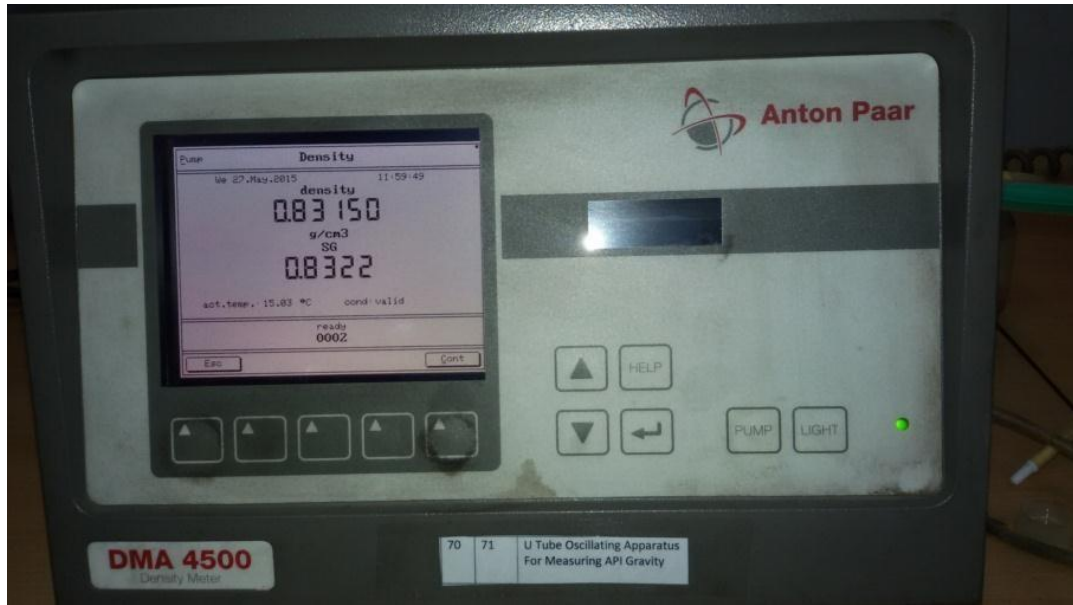
Figure 5.4 - Density Meter showing density and specific gravity for blend B-10
