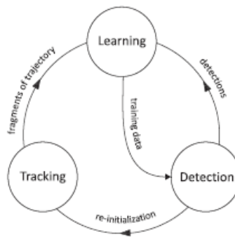
Fig. 3.1 Block diagram of TLD framework [1]
