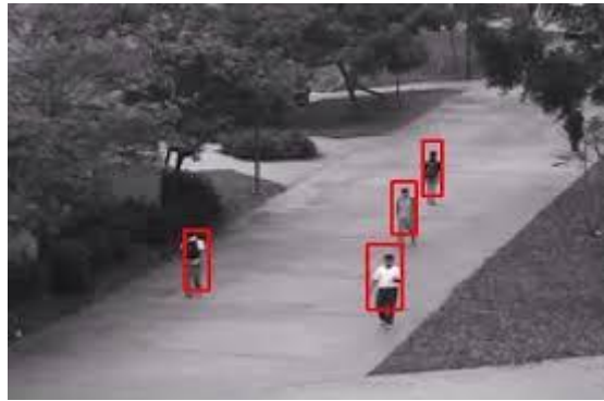
Fig. 5.8 Example of human detection through HOG
