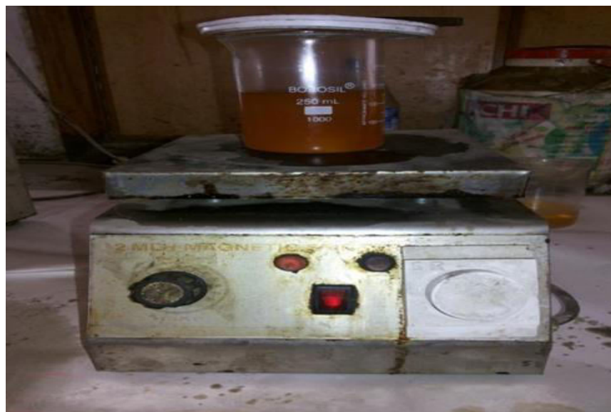
Fig. 3.1 Solution of catalyst, alcohol in WCO
