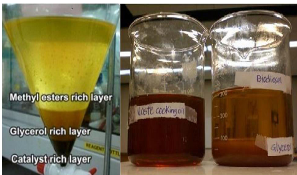
Fig. 3.2 Separation process WCO
