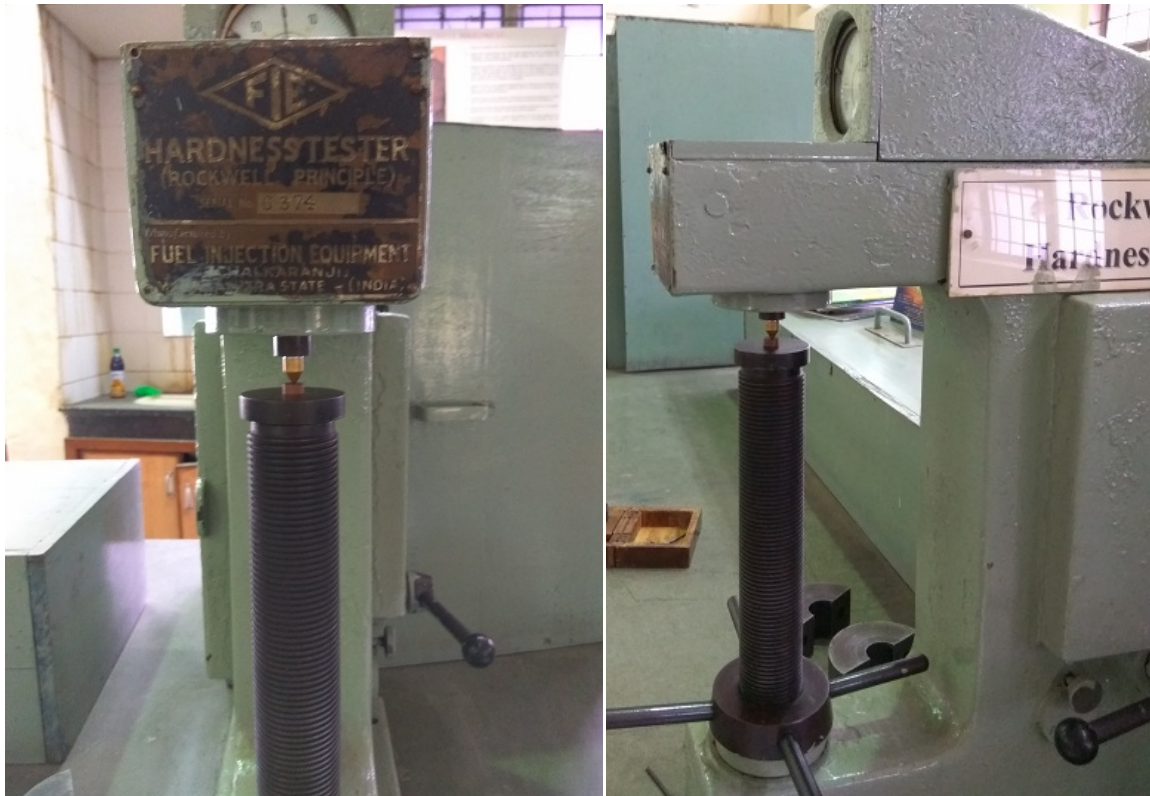
Fig 4.1 Rockwell hardness testing machine at mechanical department, DTU
