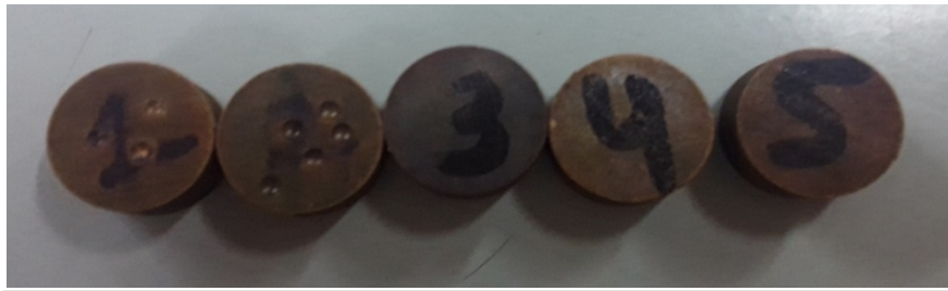
Fig 3.15 Hardness Test Specimens
