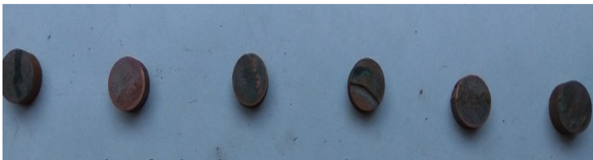
Fig 4.2 Specimen for the hardness test
