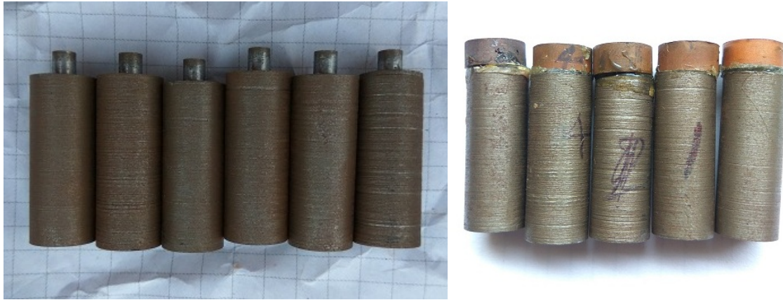
Fig 4.6 Mild steel holding pin for wear test
