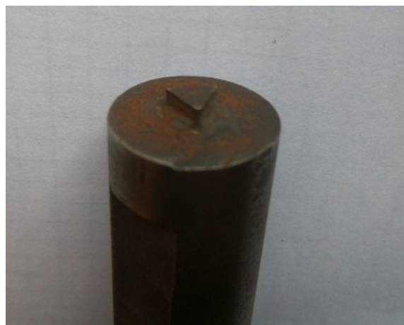
Fig 3.8 Triangular Pin tool
