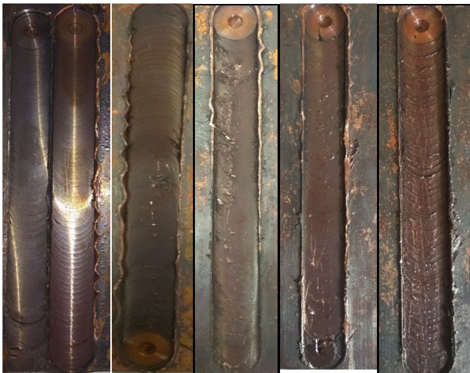
Fig 3.11 FSP Sample after Processing
