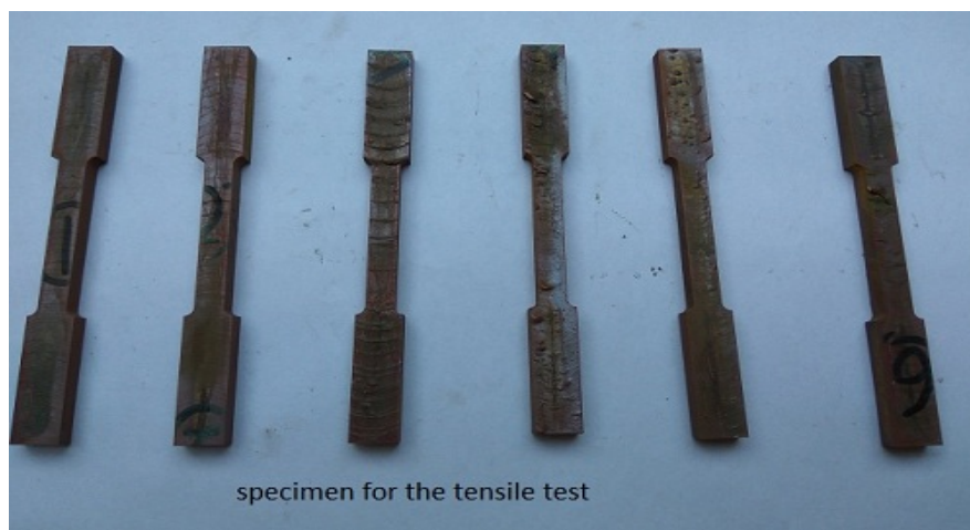
Fig 3.13 Tensile test specimens
