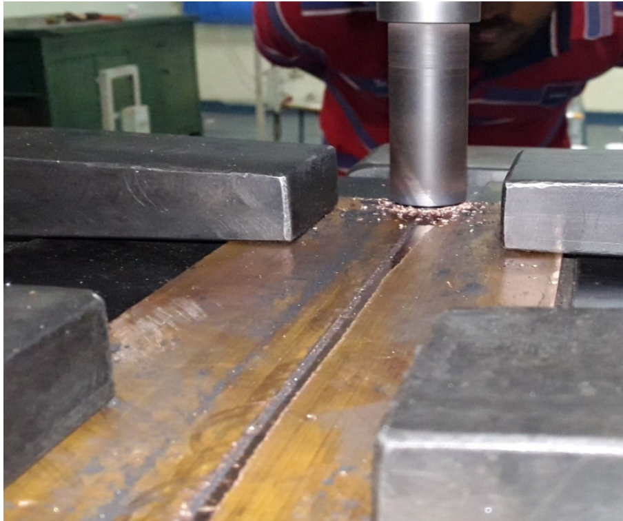
Fig 3.9 Closing of the groove by flat pin tool
