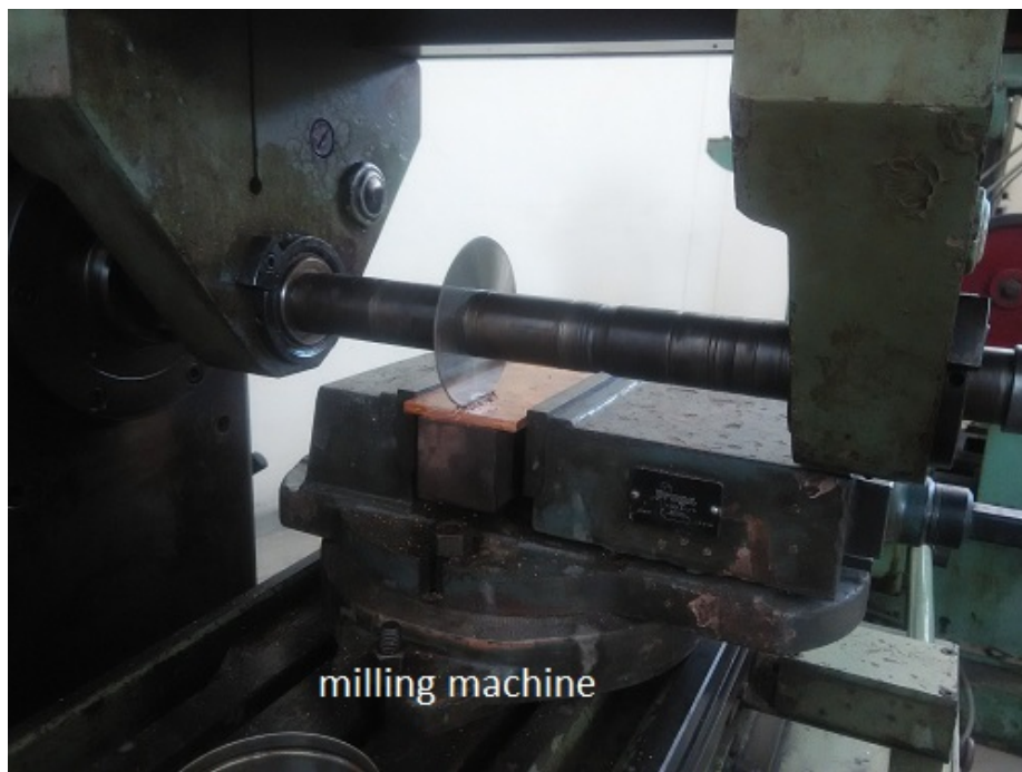
Fig 3.3 Groove cutting on the Milling machine
