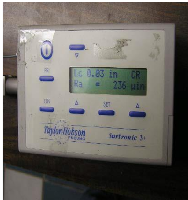
Figure12: a taylsurf instrument by taylor hobson surtronic 3+ at metrology lab, DTU
