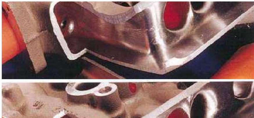
Figure 6: Intake manifold after manual AFM processing [9]
