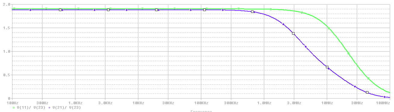
Fig.3.12. Frequency response of simple Amplifier using CDDOBA
