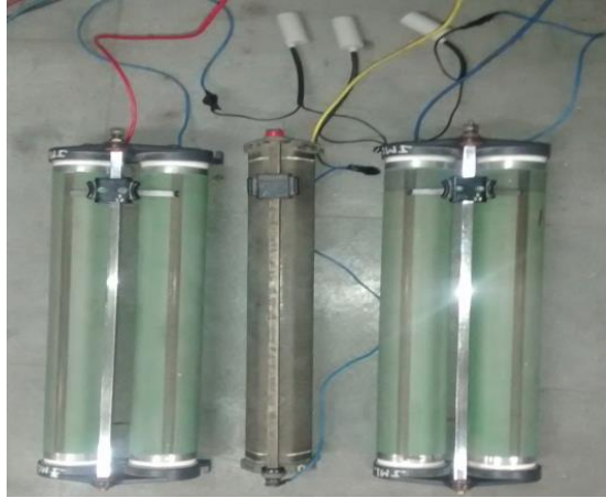
Fig. 3.16 Development of resistive capacitive (R-C) ripple filters
