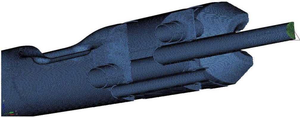
Fig. 4.11b: Section view of surface mesh of sample muffler
