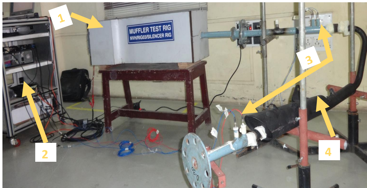
1-Speaker 2- DAQ & Amplifier 3- Microphones 4- Muffler under test
