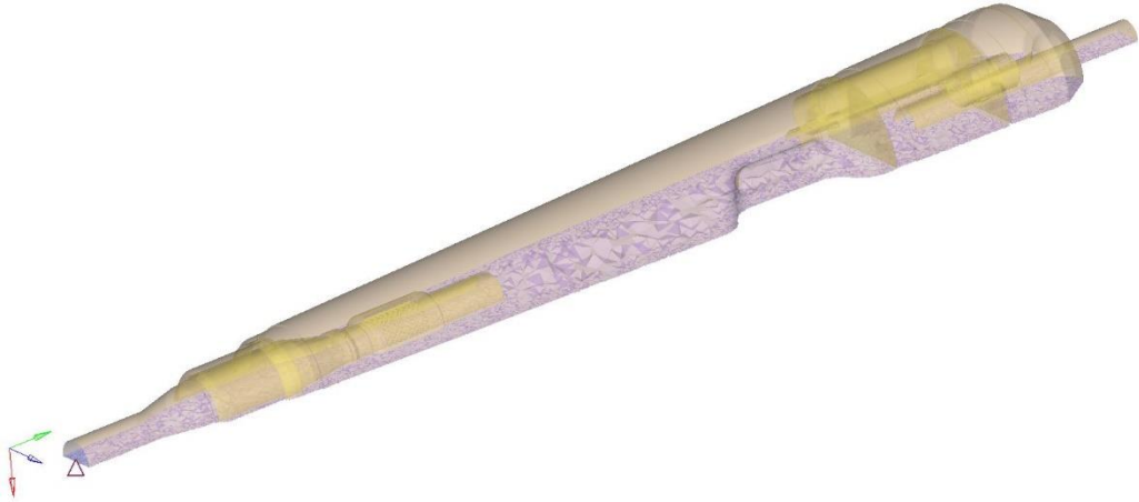
Fig. 4.11d: Transparent view of volume mesh of sample muffler
