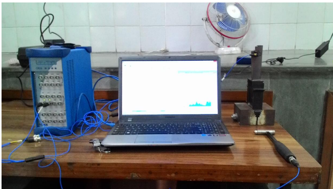
Fig.1.12. Experimental Modal Testing of gas turbine blade.
