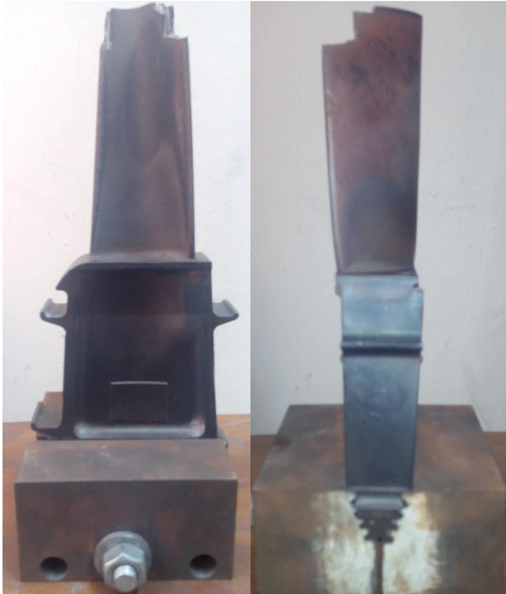
Fig. 5.7. IN738 LP-1 failed gas turbine blade
