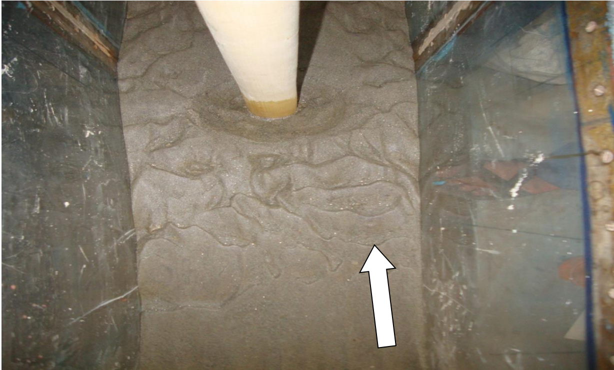
Figure: 5.5 Scour around cylindrical pier at discharge (Q)=4.08 \cdot 10^{-3} \text{ m}^3/\text{s}
