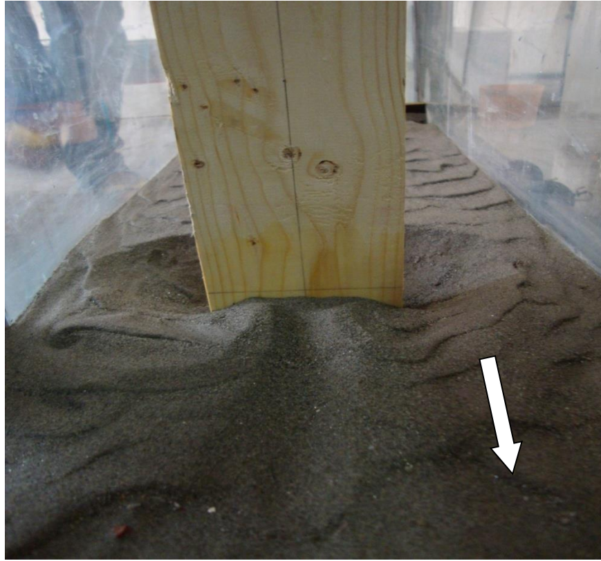
Figure: 5.24 Scour around rectangular pier at downstream side across the flow ( \Theta=90^{\circ} )
