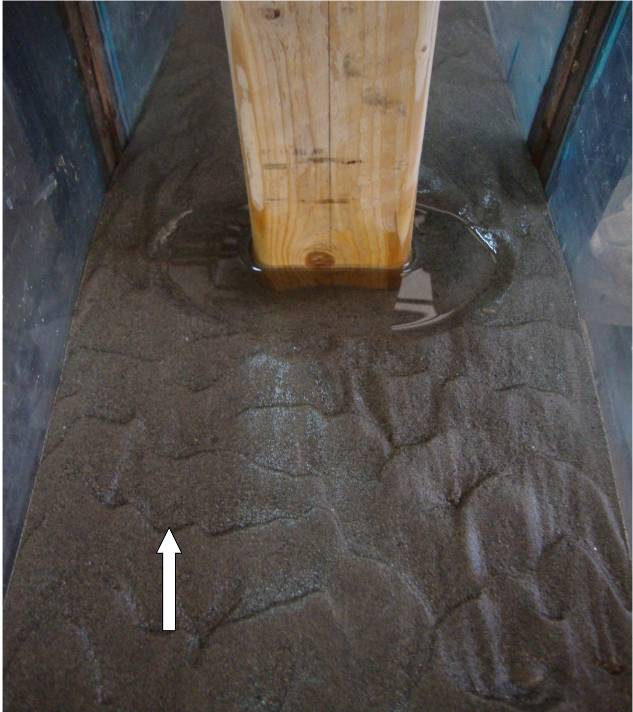
Figure: 5.13 Scour around round-nose pier at upstream side across the flow ( \Theta=90^0 )
