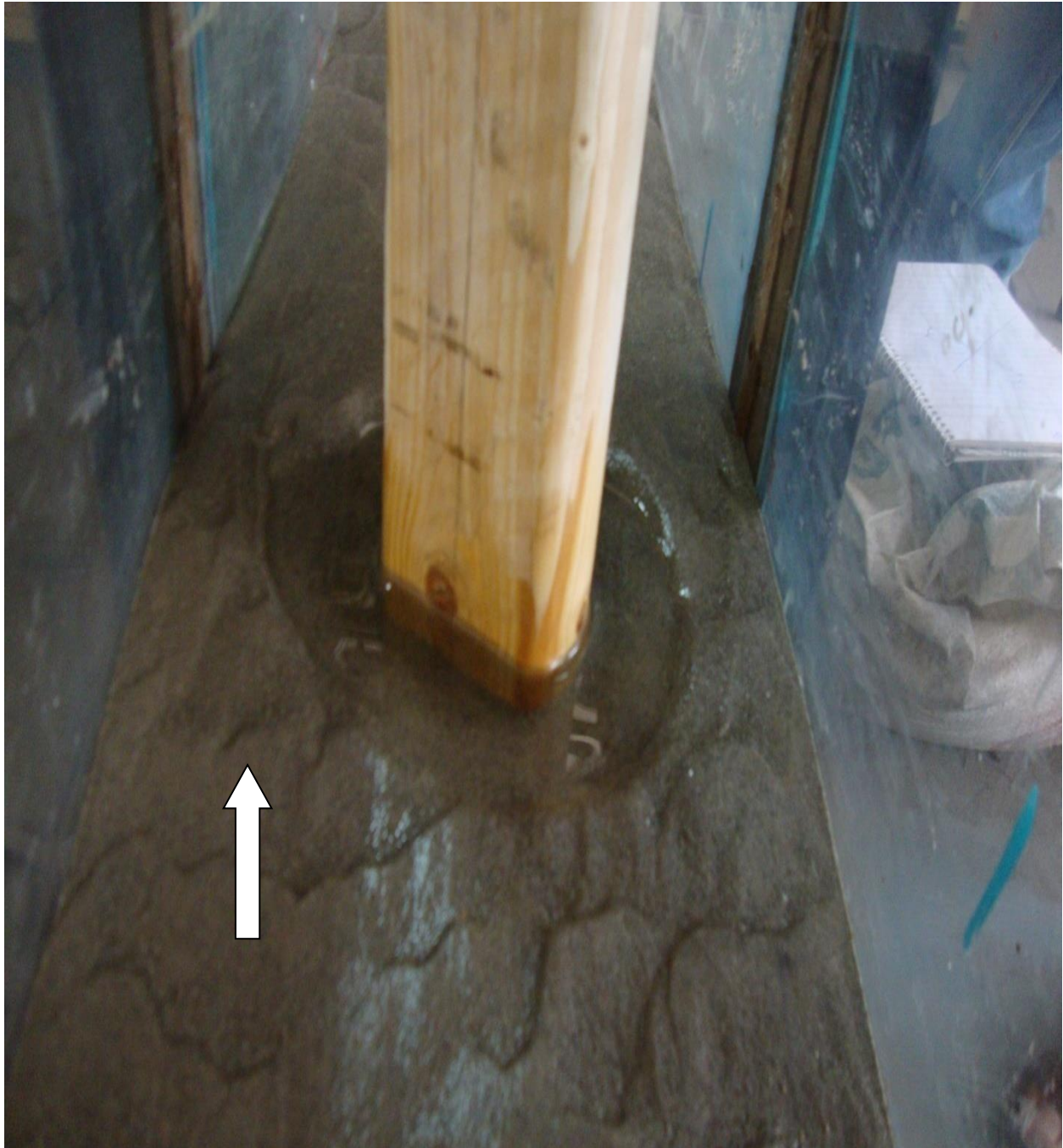
Figure: 5.12 Scour around round-nose pier at upstream side ( \Theta=60^\circ )
