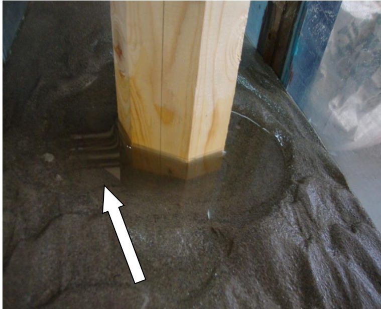
Figure: 5.20 Scour around sharp-nose pier at upstream side ( \Theta=60^{\circ} )
