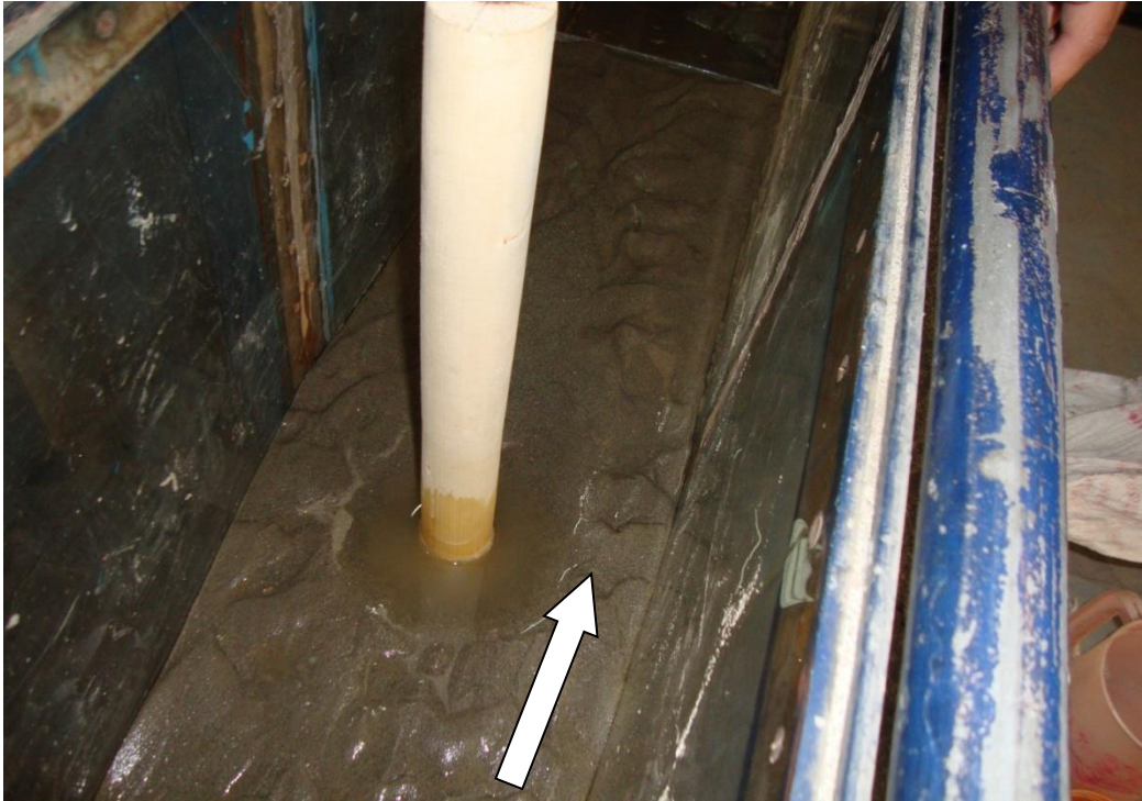
Figure: 5.3 Scour around cylindrical pier at up-stream side of flow.
