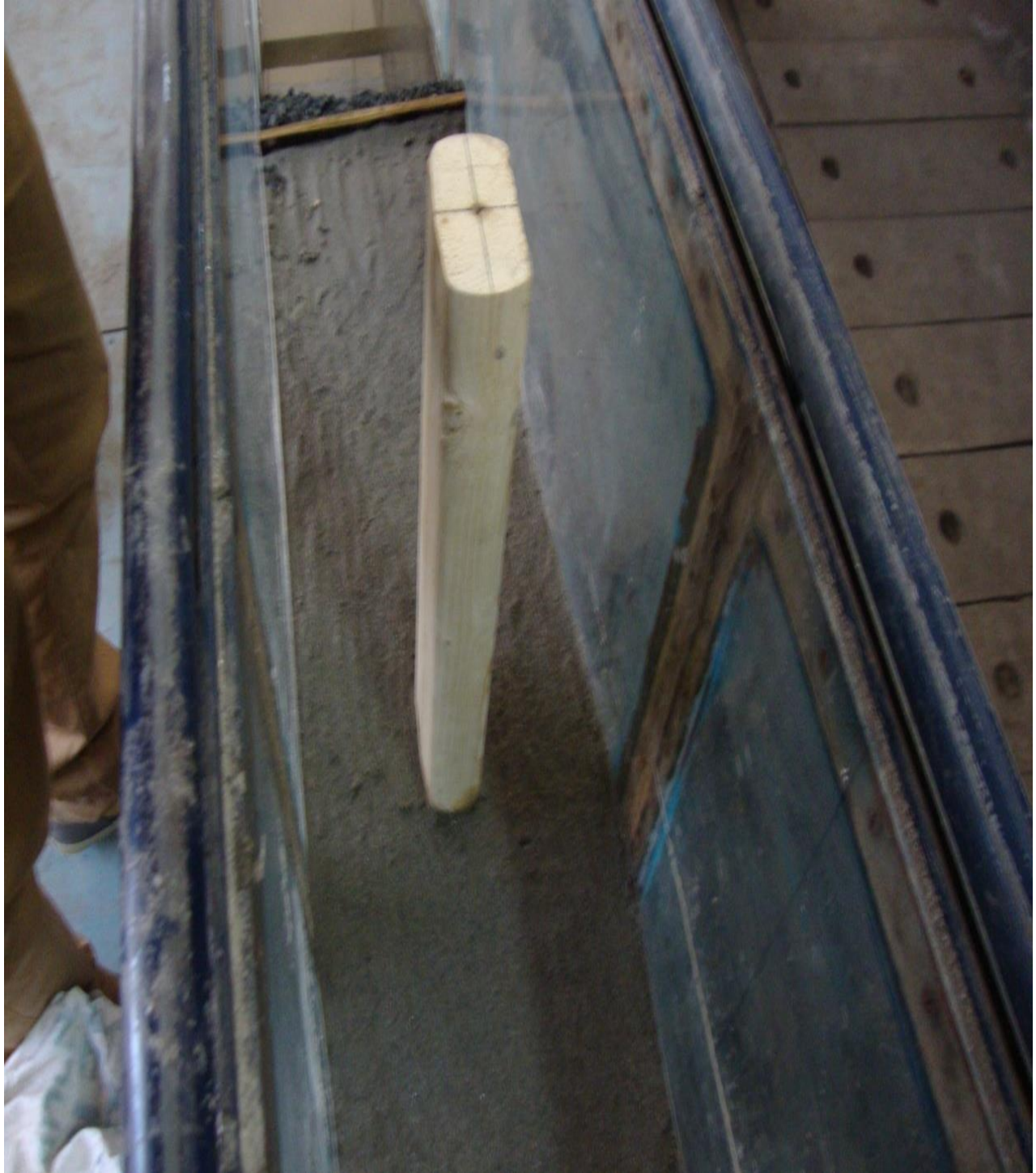
Figure 4.6: A model of round-nose pier ( l=10\text{cm} and b=5\text{cm} ) installed in a flume in laboratory
