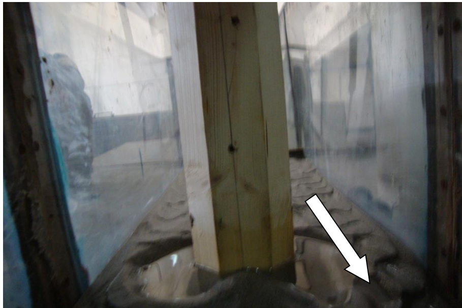
Figure: 5.21 Scour around sharp-nose pier at downstream side across the flow ( \Theta=90^{\circ} )
