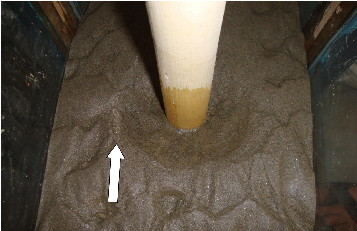
Figure: 5.4 A close look of scour around cylindrical pier at flow depth = 5.9cm
