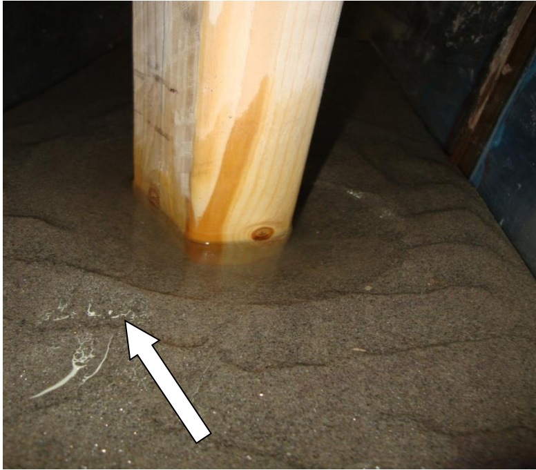
Figure: 5.9 Scour around round-nose pier at upstream side ( \Theta=30^\circ )
