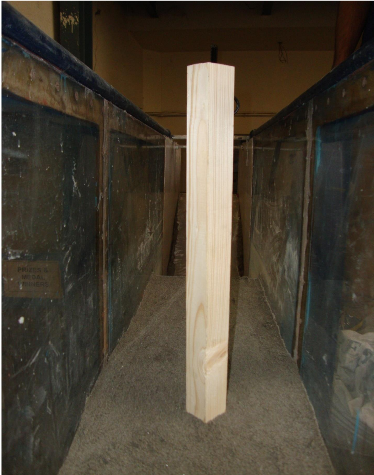
Figure 4.7: A model of sharp-nose pier ( l=10\text{cm} and b=5\text{cm} ) installed in a flume in laboratory
