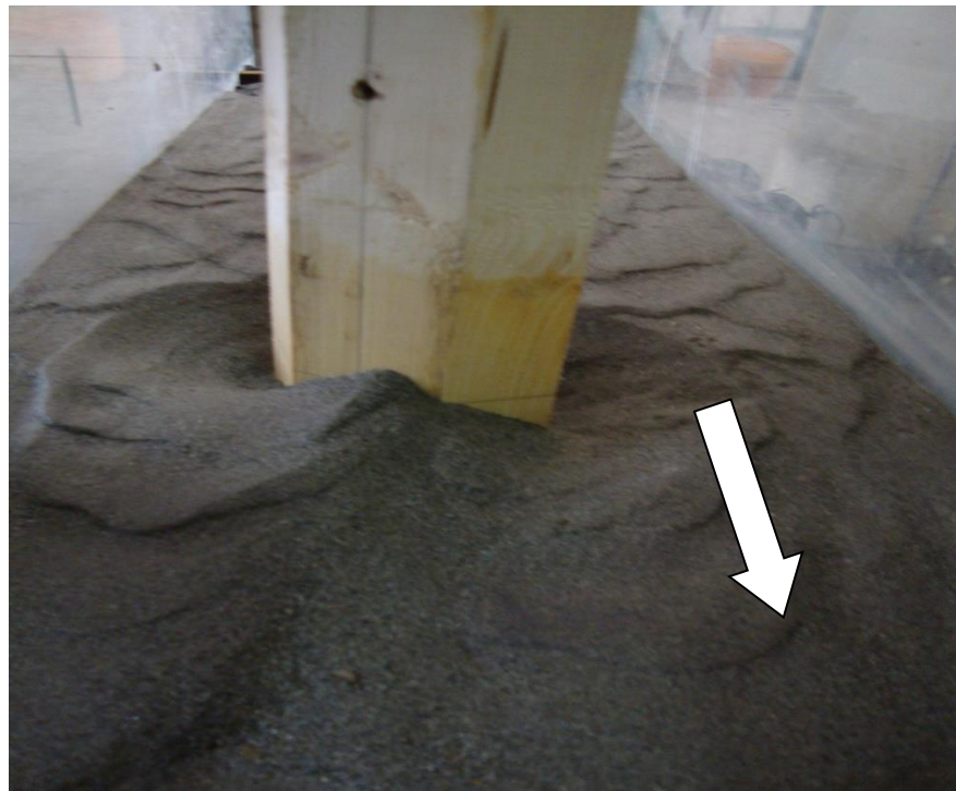
Figure: 5.19 Scour around sharp-nose pier at downstream side ( \Theta=60^\circ ) after water drained
