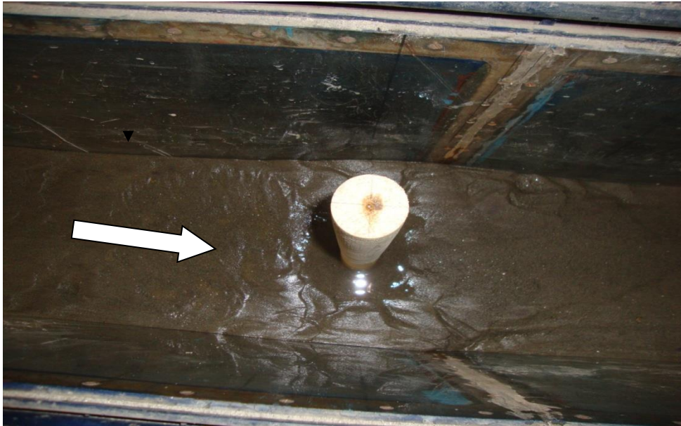
Figure: 5.1 Scour around cylindrical pier
