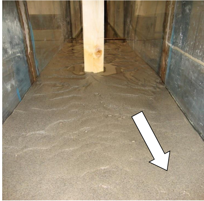
Figure: 5.16 Scour around sharp-nose pier at downstream side along the flow( \Theta=0^0 )
