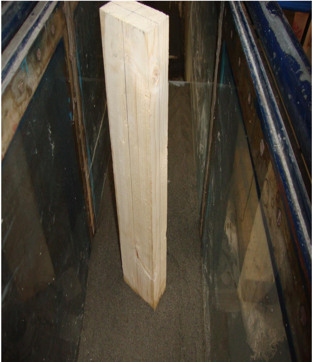
Figure 4.8: A model of rectangular pier ( l=10\text{cm} and b=5\text{cm} ) installed in a flume in laboratory
