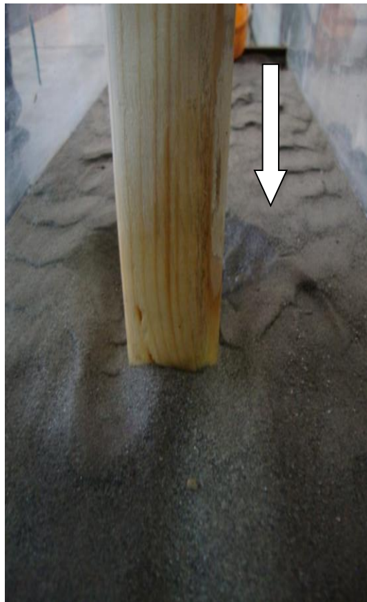
Figure: 5.8 Scour around round-nose pier at downstream side along the channel flow( \Theta=0^0 )
