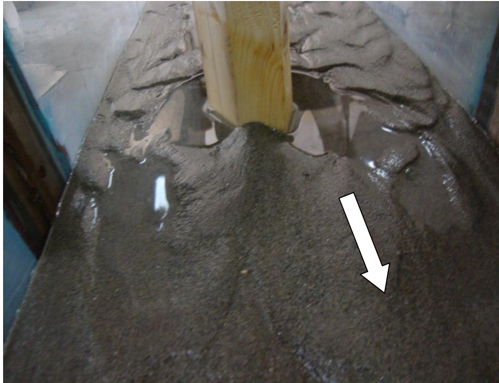
Figure: 5.17 Scour around sharp-nose pier at downstream side ( \Theta=30^0 )
