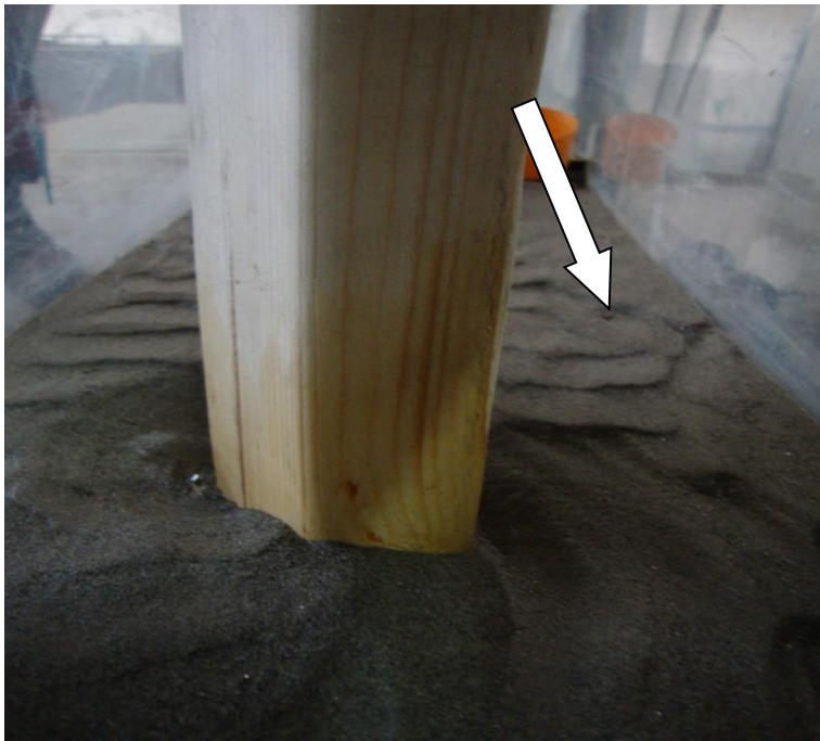
Figure: 5.10 Scour around round-nose pier at downstream side ( \Theta=30^\circ )
