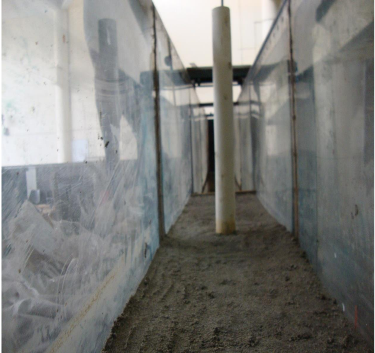
Figure 4.5: A model of cylindrical pier ( b=5\text{cm} ) installed in a flume in laboratory.
