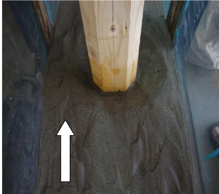
Figure: 5.22 Scour around sharp-nose pier at upstream side across the flow ( \Theta=90^0 )
