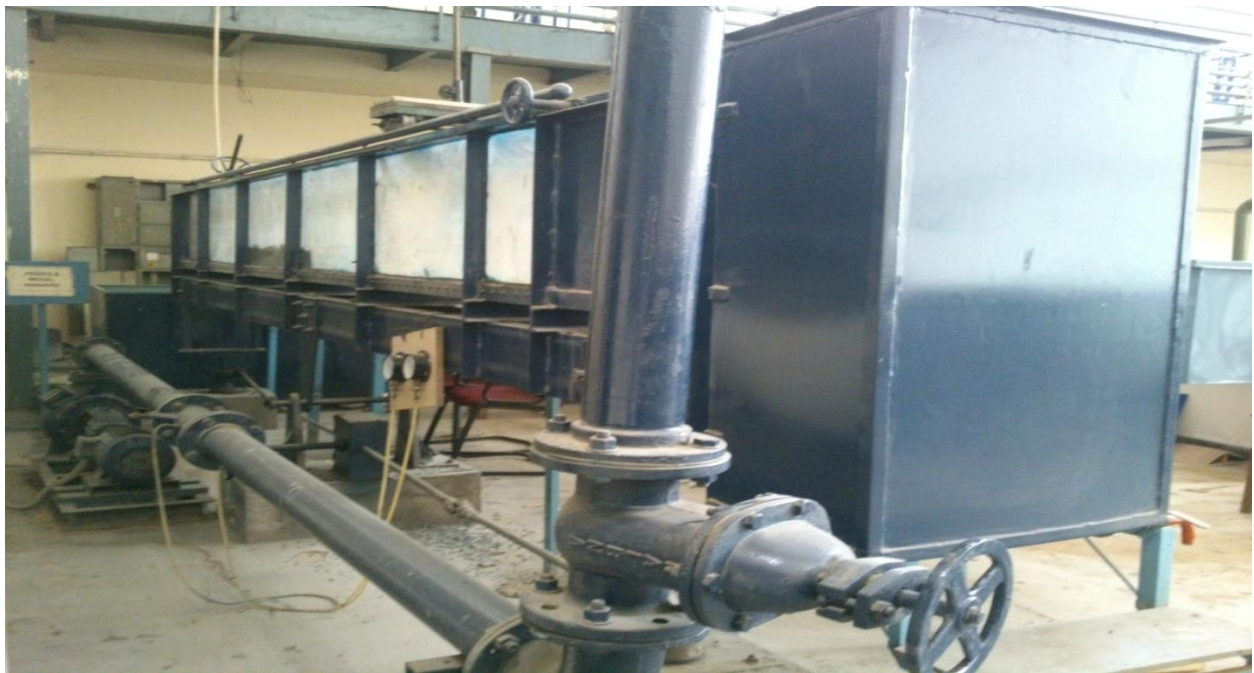
Figure: 4.2 A hydraulic tilting flume on which all experiments were performed in laboratory.
