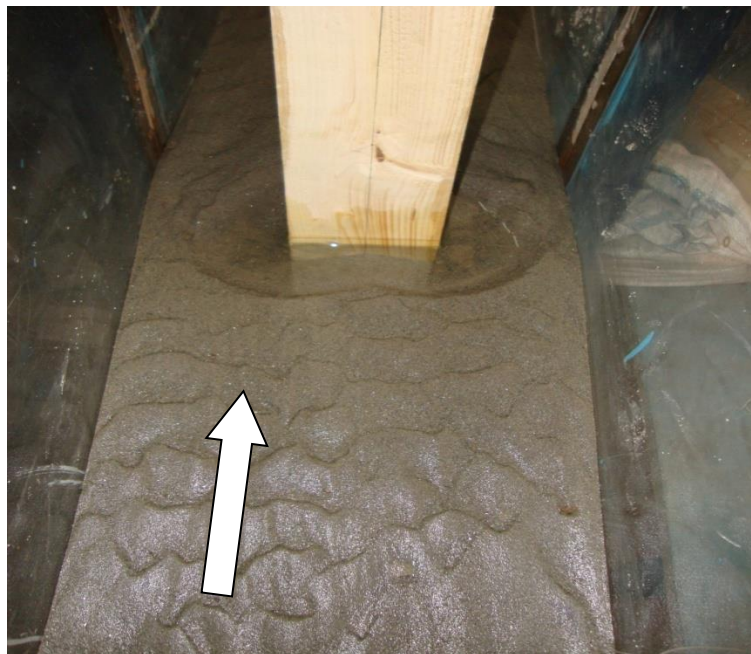
Figure: 5.23 Scour around rectangular pier at upstream side across the flow ( \Theta=90^0 )
