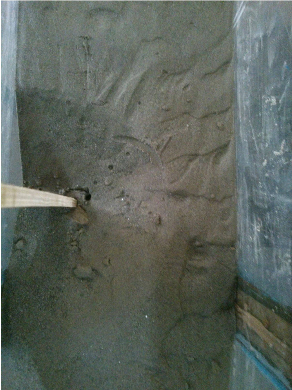
Figure 5.1 Normal spur dike after scouring occurs ( \Theta=90^\circ )
