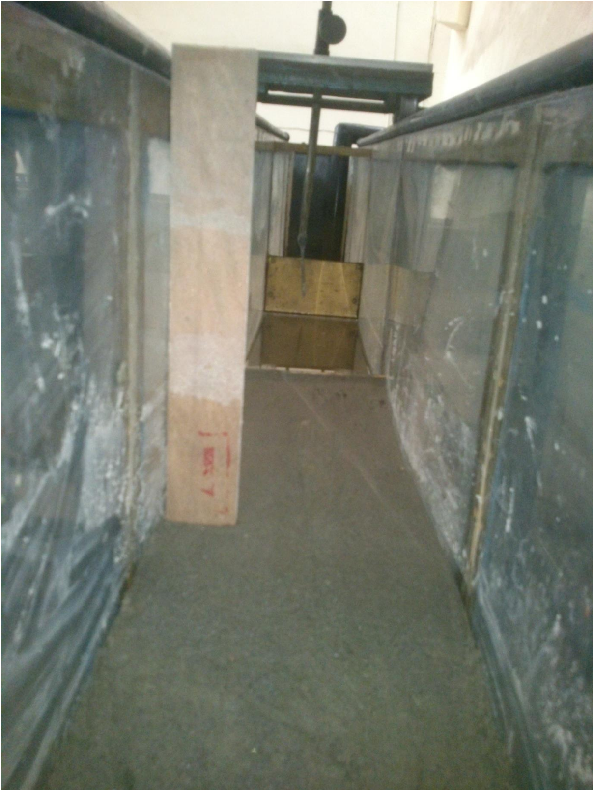
Figure 4.4 Normal dike before scouring ( \Theta=60^\circ ).
