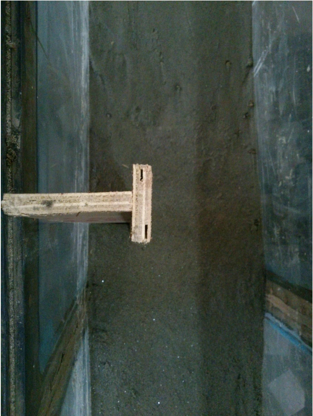
Figure 4.6 T shaped spur dike before scouring ( \Theta=90^\circ ).
