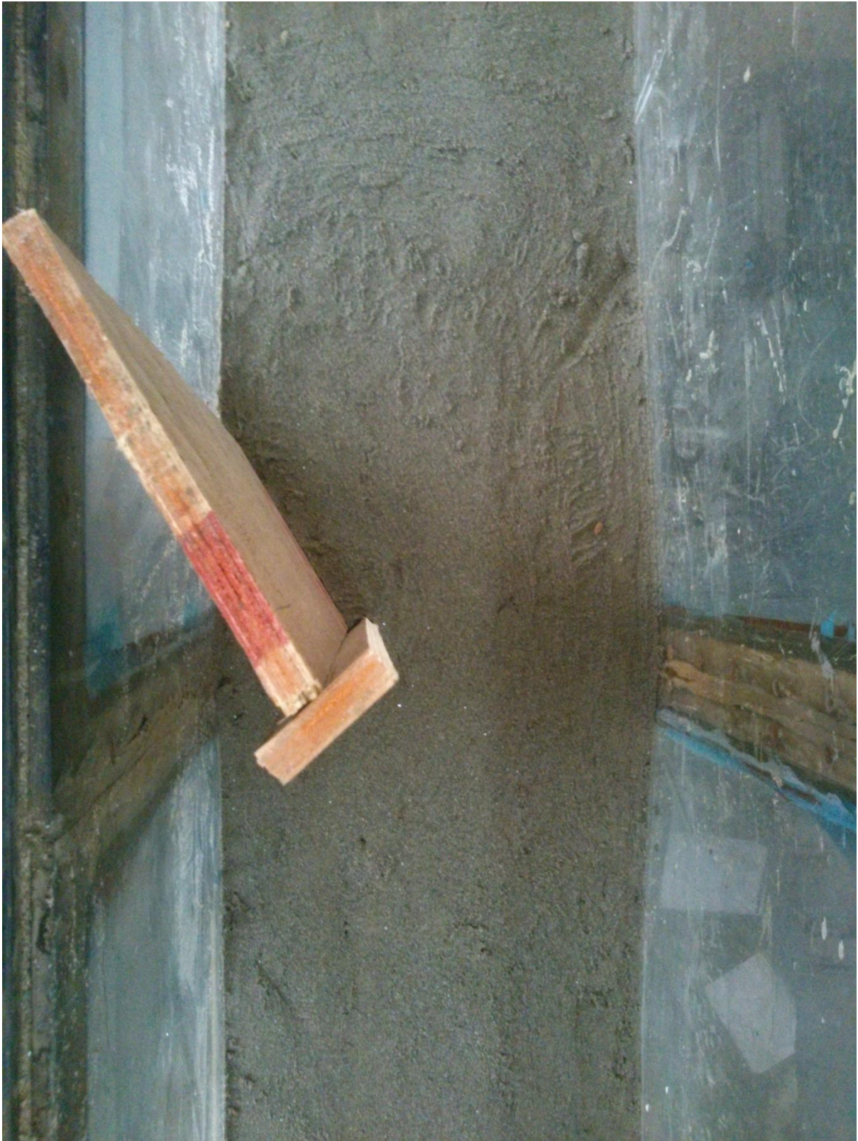
Figure 4.8 T shaped spur dike before scouring ( \Theta=30^\circ ).
