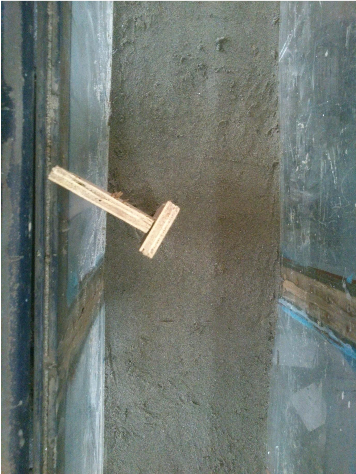
Figure 4.7 T shaped spur dike before scouring ( \Theta=60^\circ ).
