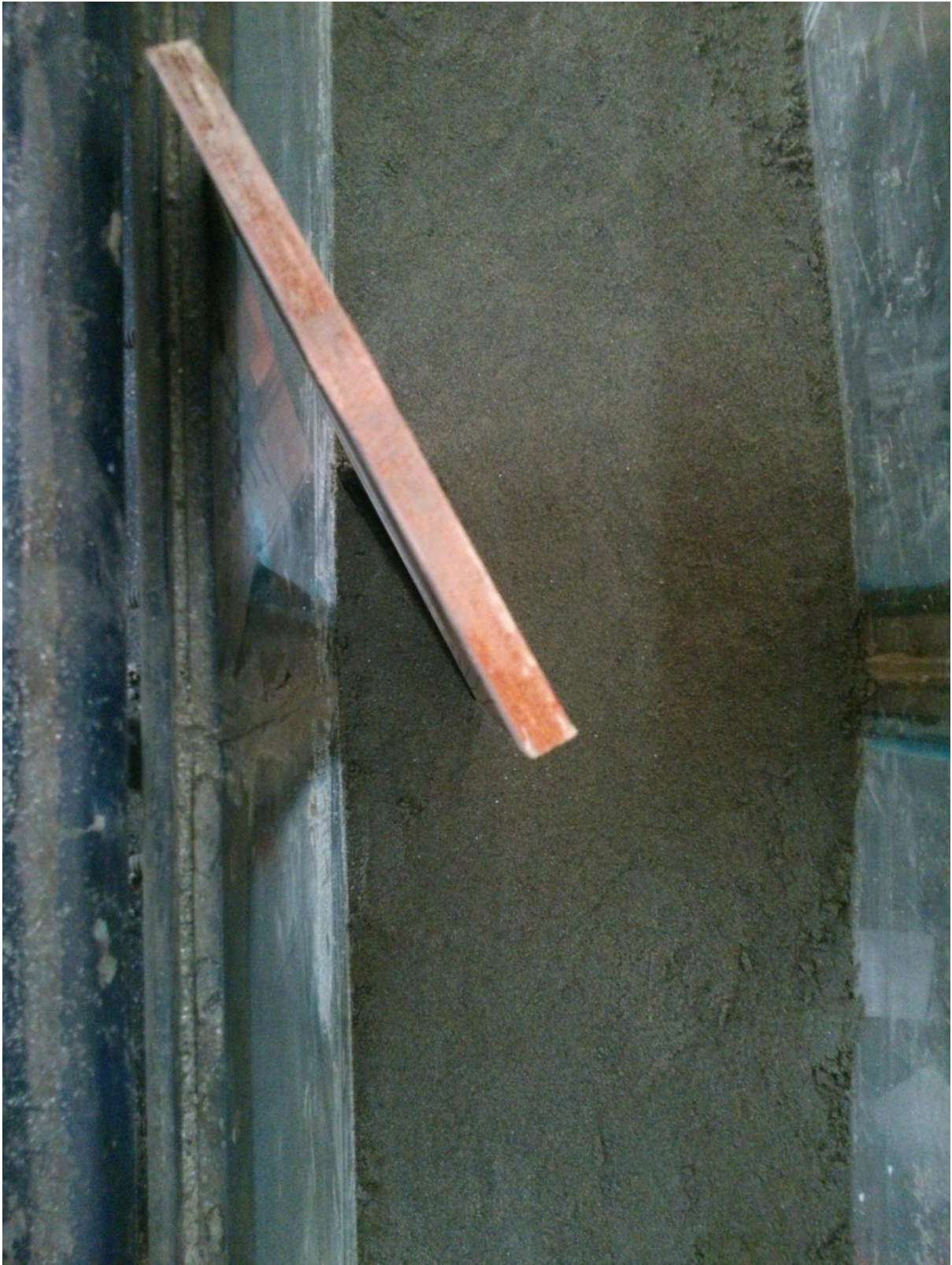
Figure 4.5 Normal spur dike before scouring ( \Theta=30^\circ ).
