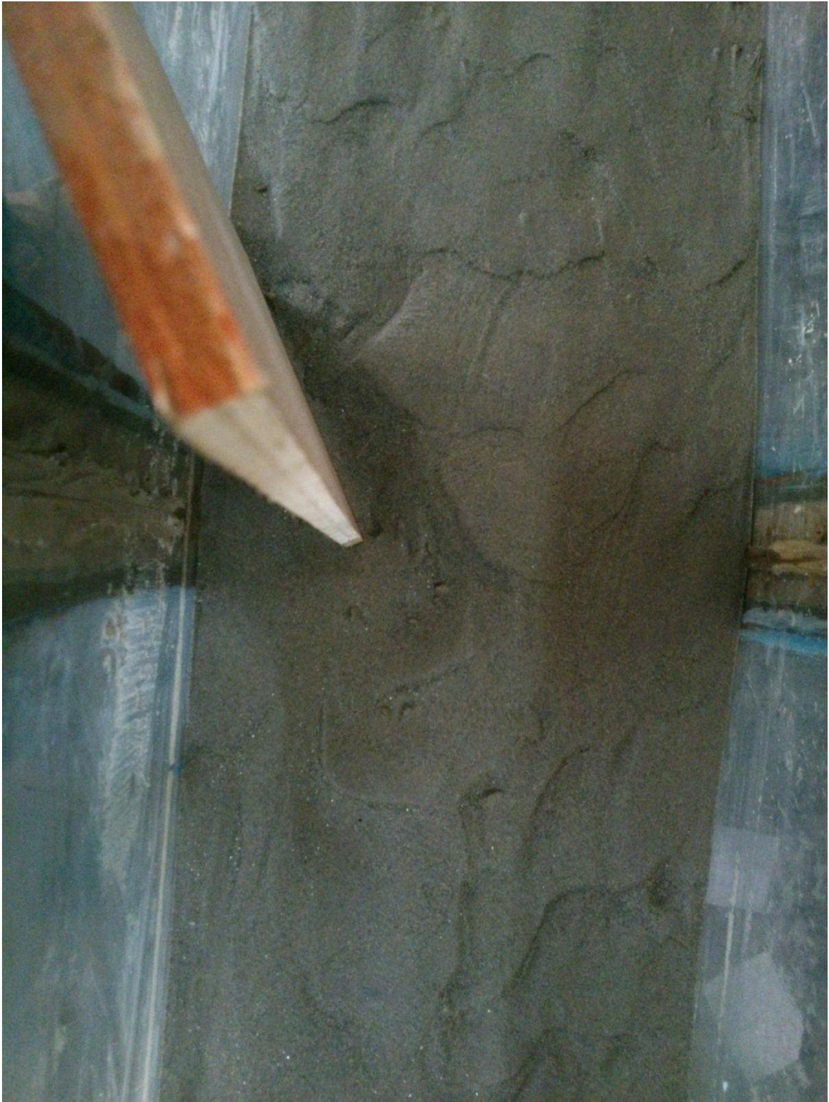
Figure 5.3 Normal spur dike after scour occurs ( \Theta=30^\circ )
