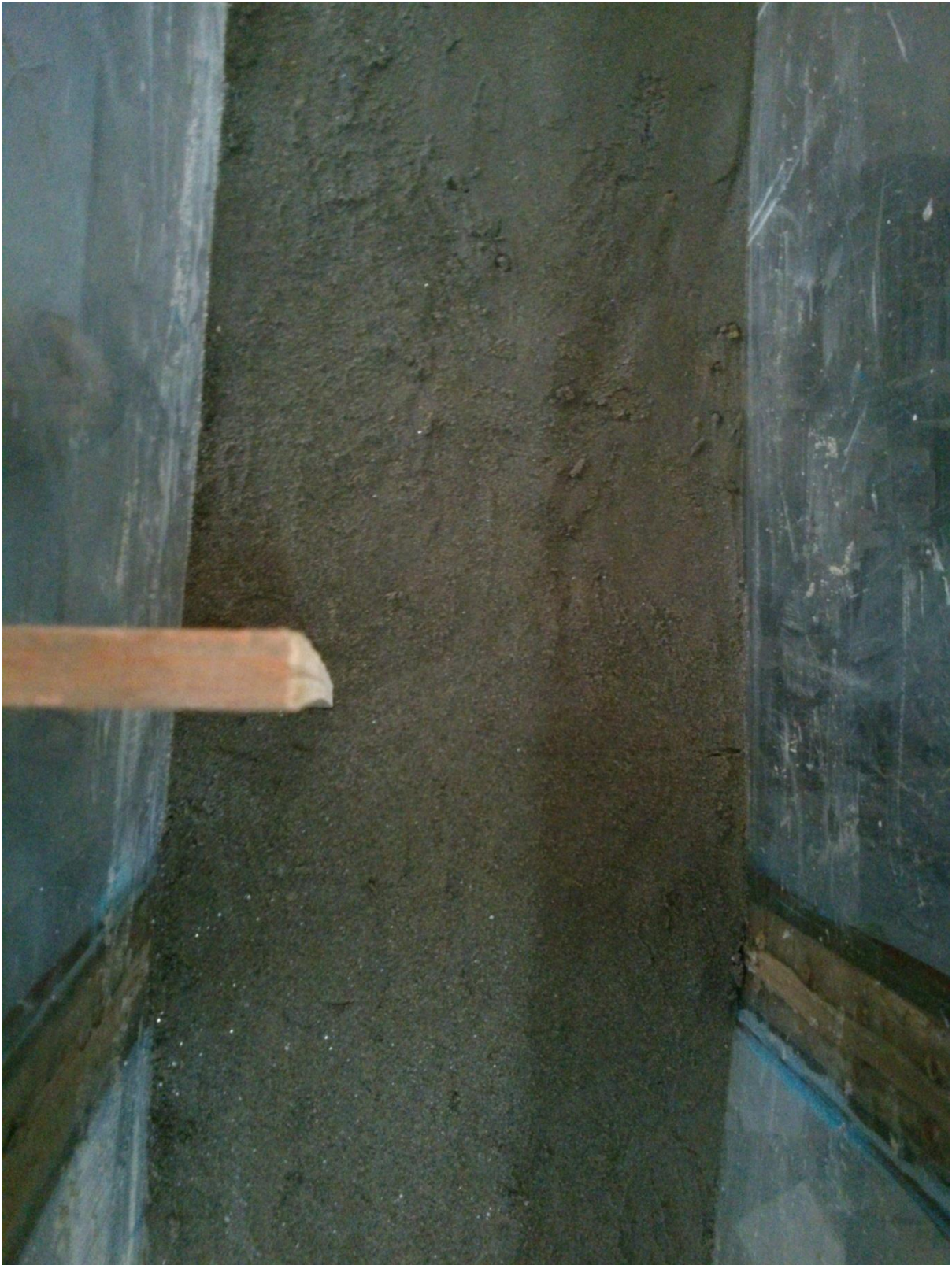
Figure 4.3 normal spur dike before scouring ( \Theta=90^\circ ).
