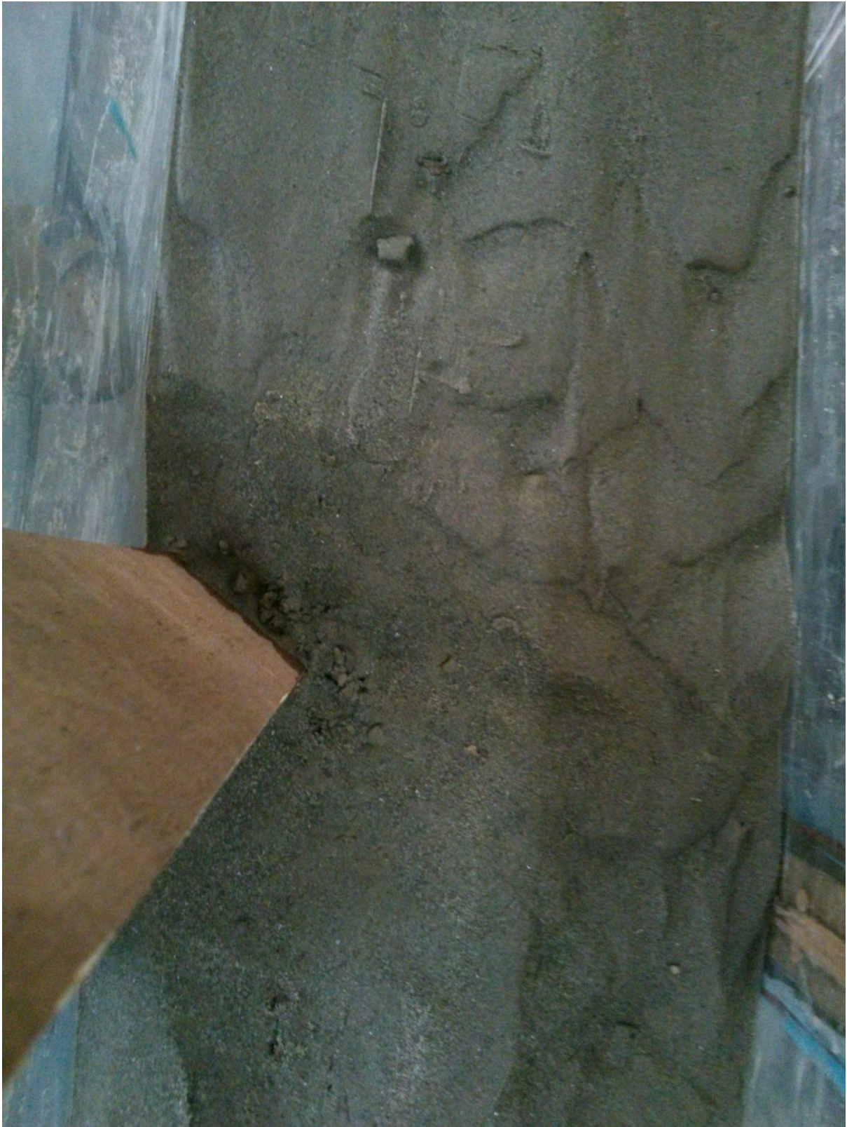
Figure 5.2 Normal spur dike after scour occurs ( \Theta=60^\circ )
