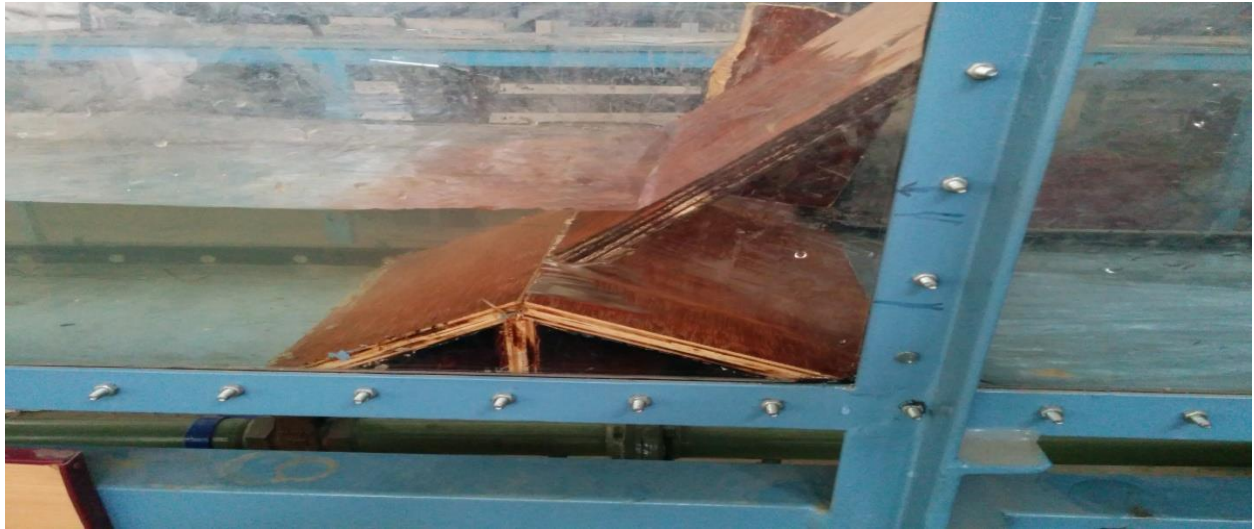
Figure 20: when a sluice gate with sharp edge lip is inclined in the opposite direction of flow with a sill/hump of 7.5 cm.
