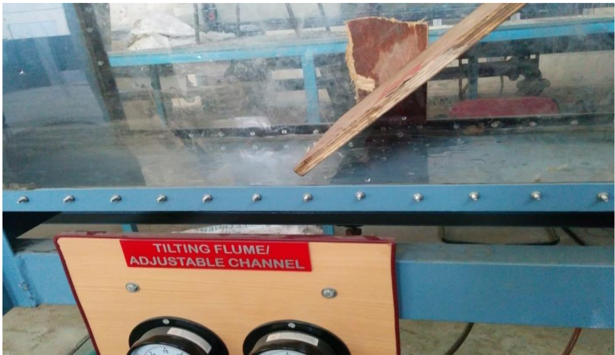
Figure 11: when a sluice gate with horizontal edge is inclined in the opposite direction of flow without a sill/hump.
