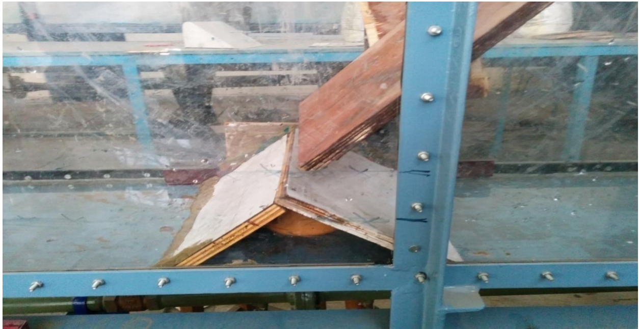
Figure 22: when a sluice gate with sharp edge is inclined in the opposite direction of flow on the the sill of 11.5 cm.
