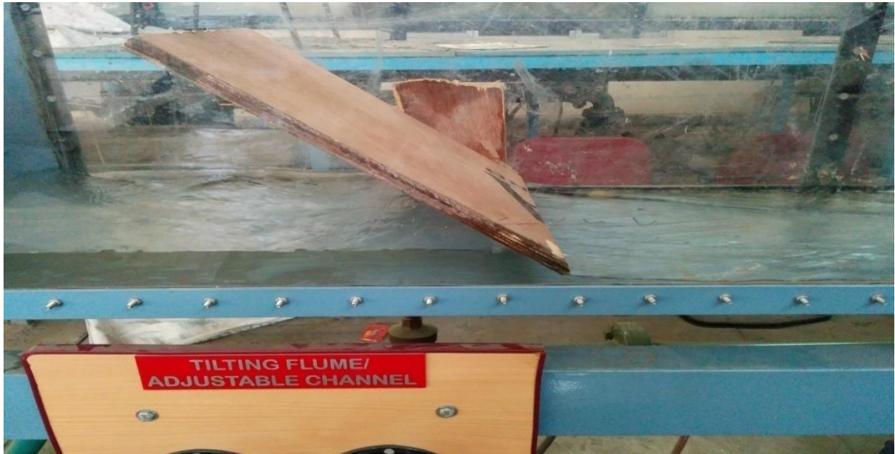
Figure 15: when a sluice gate with sharp edge lip is inclined in the direction of flow without a sill/hump.
