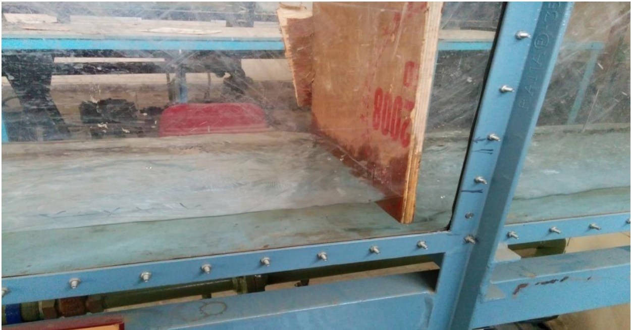
Figure 3: when a sluice gate with horizontal edge is installed vertically without a sill/hump.
