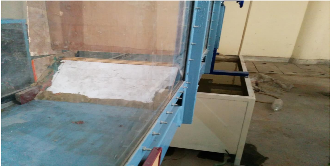
Figure 6: when a sluice gate with horizontal edge is placed vertically on the the sill of 11.5 cm.
