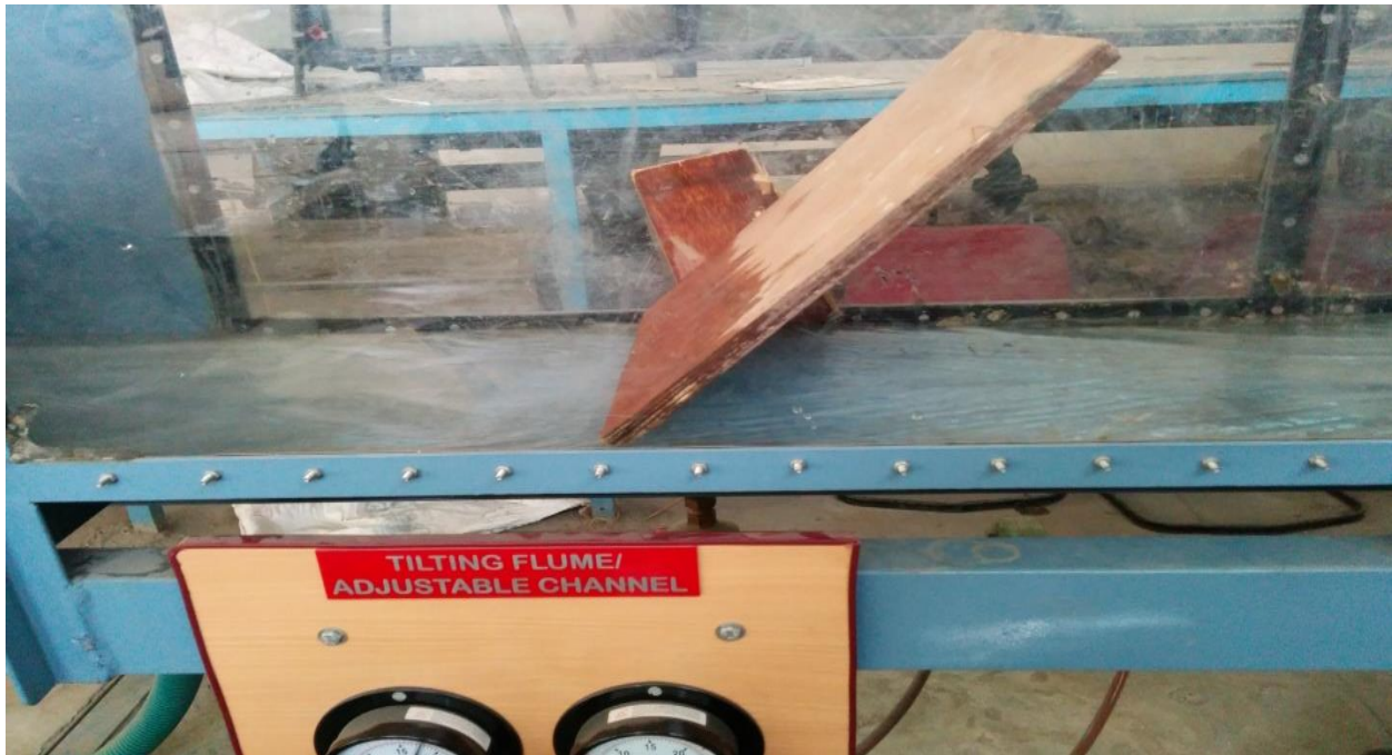
Figure 19: when a sluice gate with sharp edge lip is inclined in the opposite direction of flow without a sill/hump.
