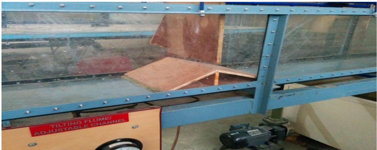
Figure 5: when a sluice gate with horizontal edge is placed vertically on the the sill of 10 cm.
