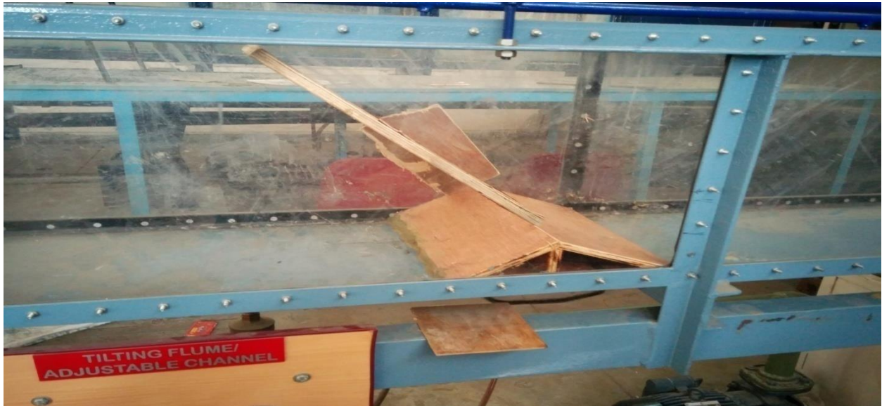
Figure 8: when a sluice gate with horizontal edge is inclined in the direction of flow with a sill/hump of 7.5 cm.
