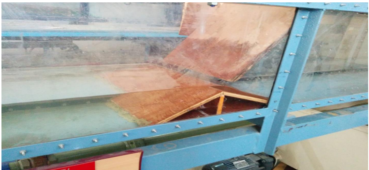
Figure 21: when a sluice gate with sharp edge is inclined in the opposite direction of flow on the the sill of 10 cm.
