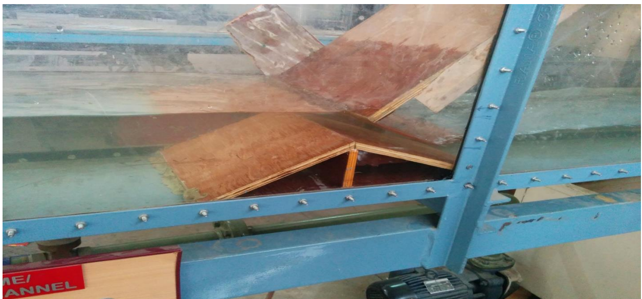
Figure 13: when a sluice gate with horizontal edge is inclined in the opposite direction of flow on the the sill of 10 cm.
