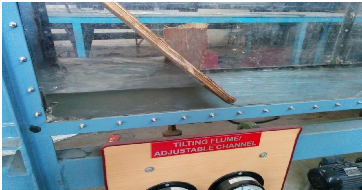
Figure 7: when a sluice gate with horizontal edge is inclined in the direction of flow without a sill/hump.
