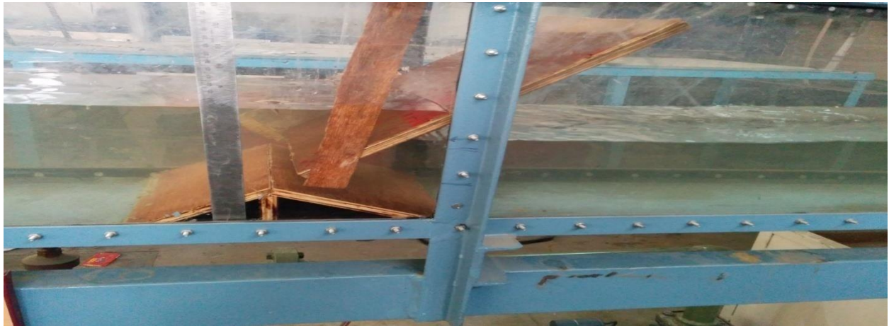
Figure 12: when a sluice gate with horizontal edge is inclined in the opposite direction of flow with a sill/hump of 7.5 cm.
