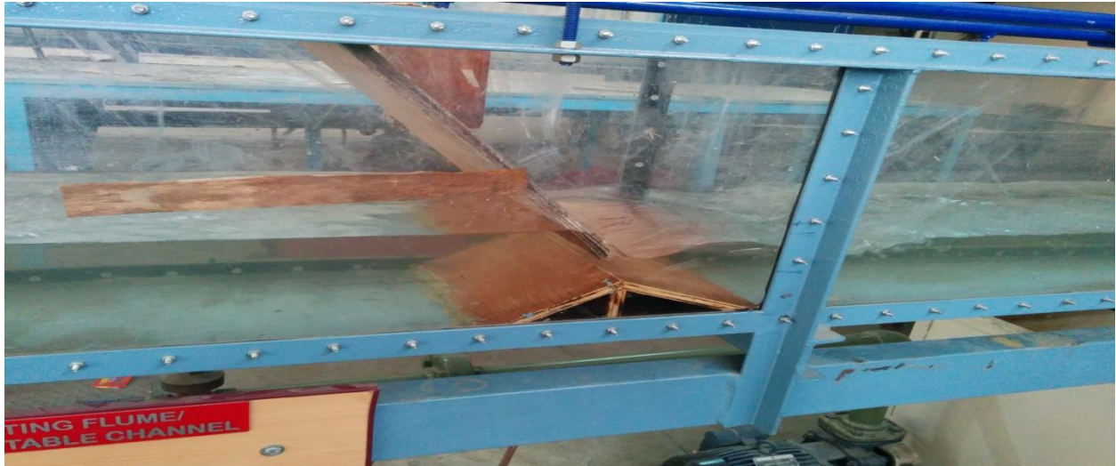
Figure 16: when a sluice gate with sharp edge lip is inclined in the direction of flow with a sill/hump of 7.5 cm.
