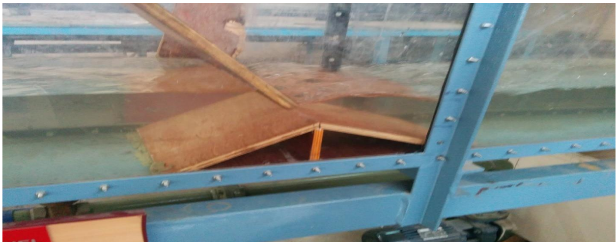
Figure 9: when a sluice gate with horizontal edge is inclined in the direction of flow on the the sill of 10 cm.
