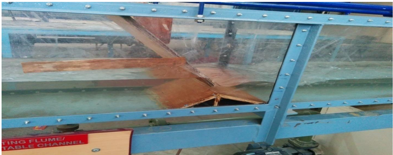
Figure 17: when a sluice gate with sharp edge is inclined in the direction of flow on the the sill of 10 cm.
