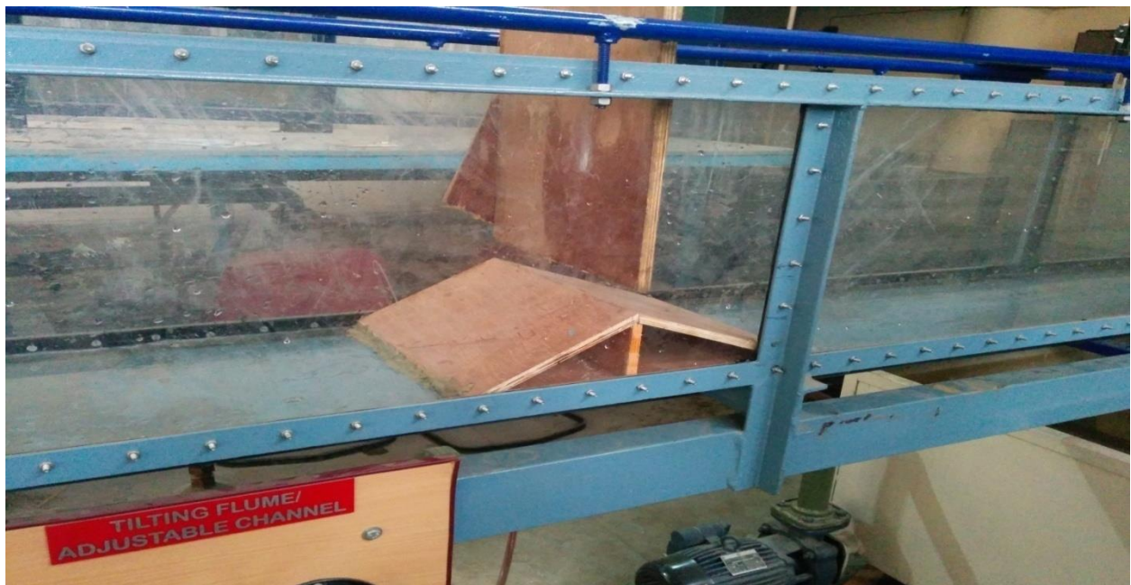
Figure-2. Representation of the sill model and sluice gate in the flume.
