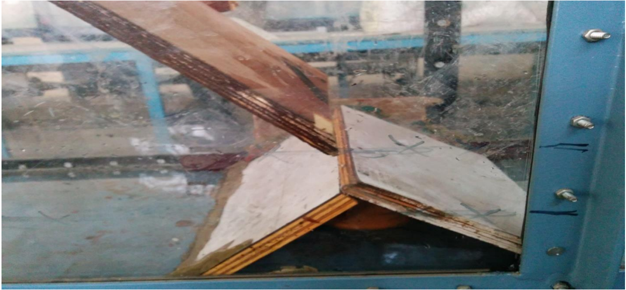
Figure 18: when a sluice gate with sharp edge is inclined in the direction of flow on the the sill of 11.5 cm.
