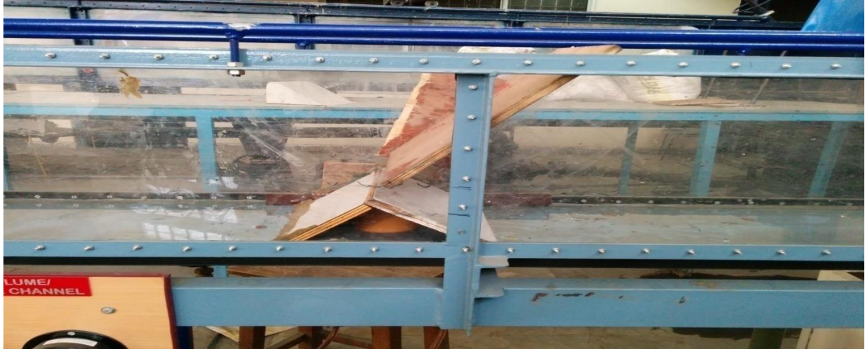
Figure 14: when a sluice gate with horizontal edge is inclined in the opposite direction of flow on the the sill of 11.5 cm.
