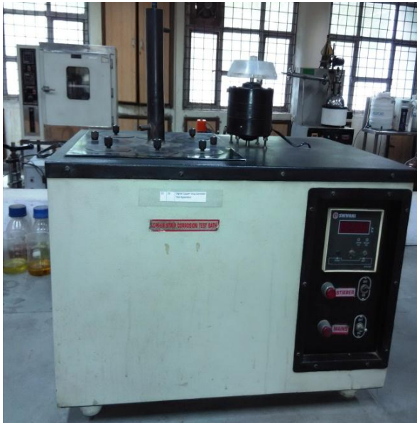
Plate 3.14: Copper Strip Corrosion Test Apparatus
