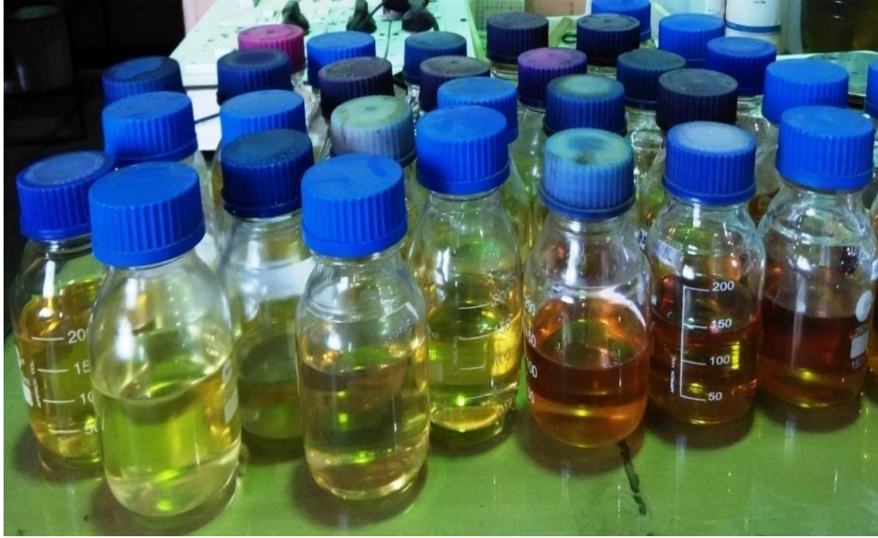
Plate 3.19 SME and KME fuel samples for storage stability test
