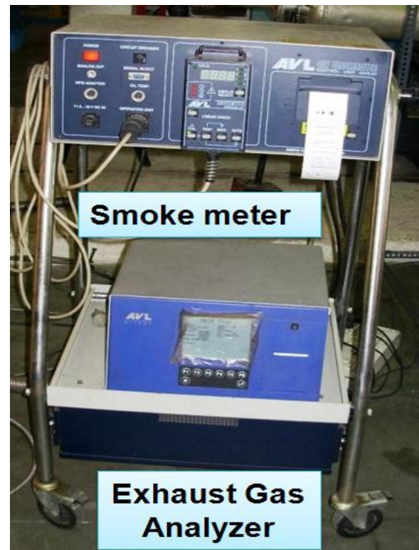
Plate 3.24 Exhaust gas analyzer and smoke meter
