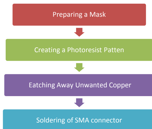
Figure 5.1: Flowchart of fabrication processes
