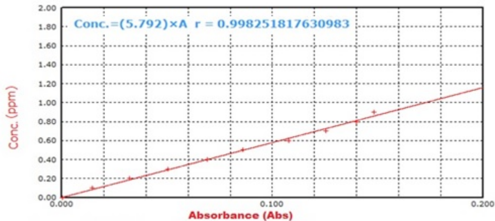
Figure 3.4: Standard curve for iron (Labtronics make Model LT-290 spectrophotometer)
