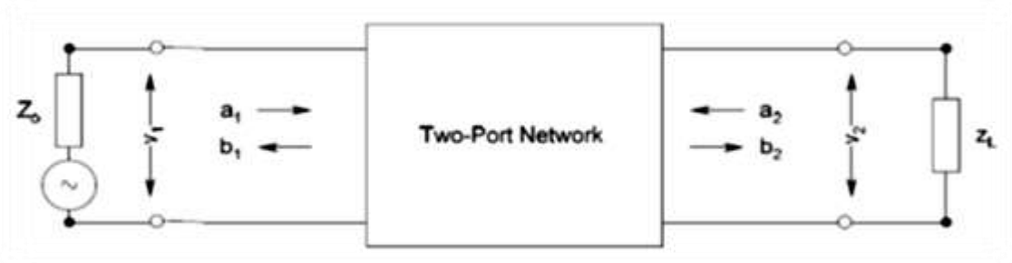
Figure 3.2: Two port network showing incident and reflected wave
