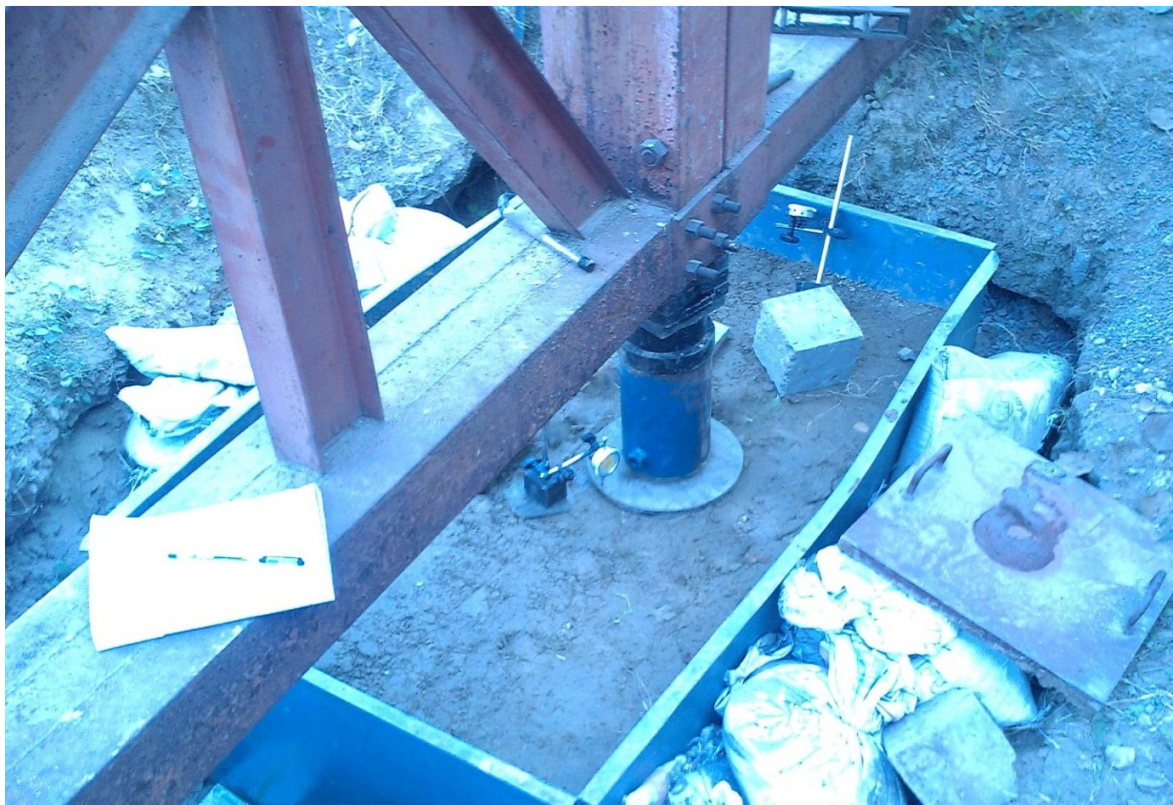
Picture 8: Loading applied on silty clay bed
