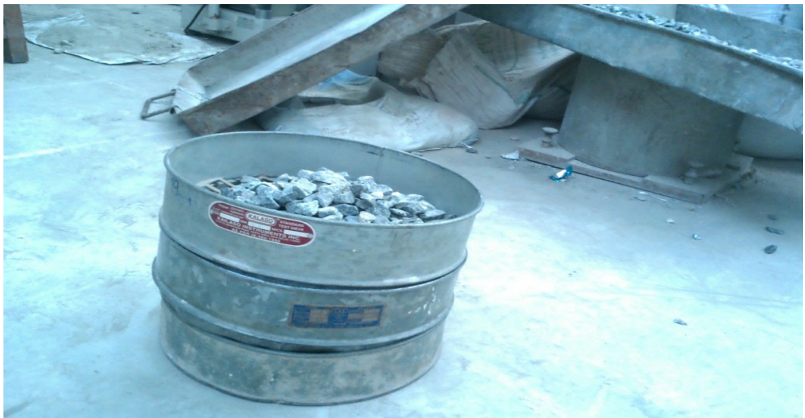
Picture 10: Sieves used for gradation of aggregates
