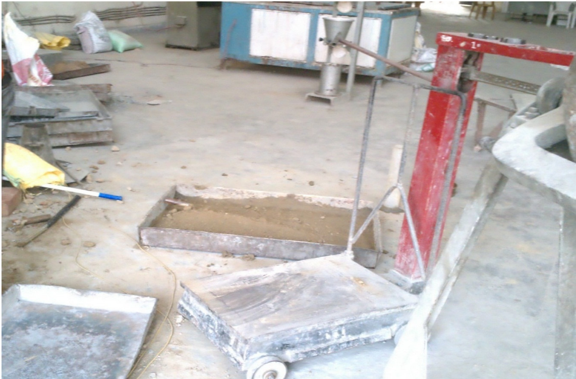
Picture 6: Mixing and weighing of soil with water in batches upto optimum moisture content
