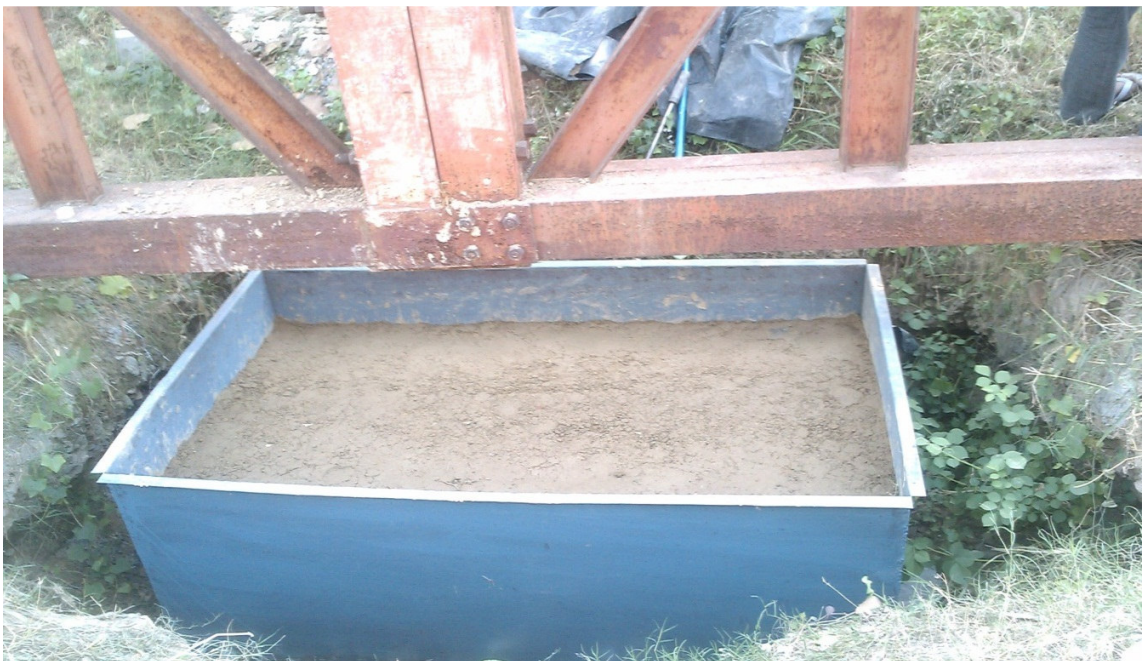
Picture 7: 1125 kilograms of soil filled in tank volume 1.5m×0.6m×0.75m
