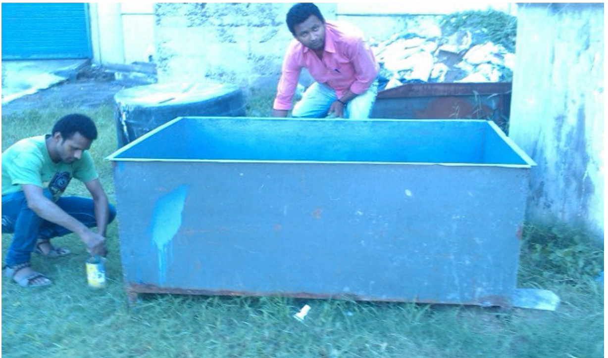
Picture 1:Rectangular tank used for soil bed preparation (1.5m×0.6m×0.9m)
