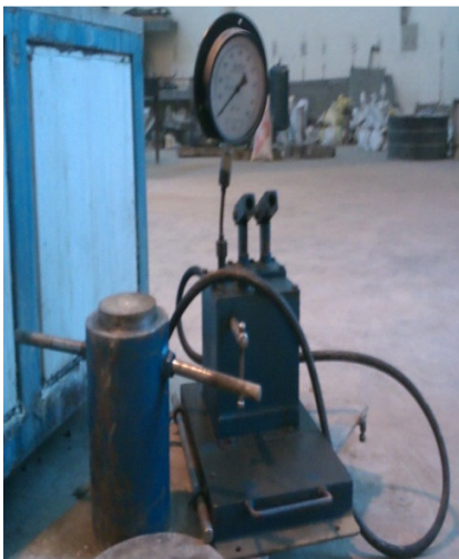
Picture 3: Hydraulic jack used for loading
