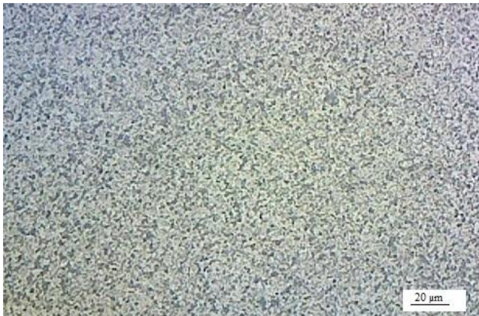
Figure No. 15 (d) Microstructure of the three pass FSPed specimen cross section
