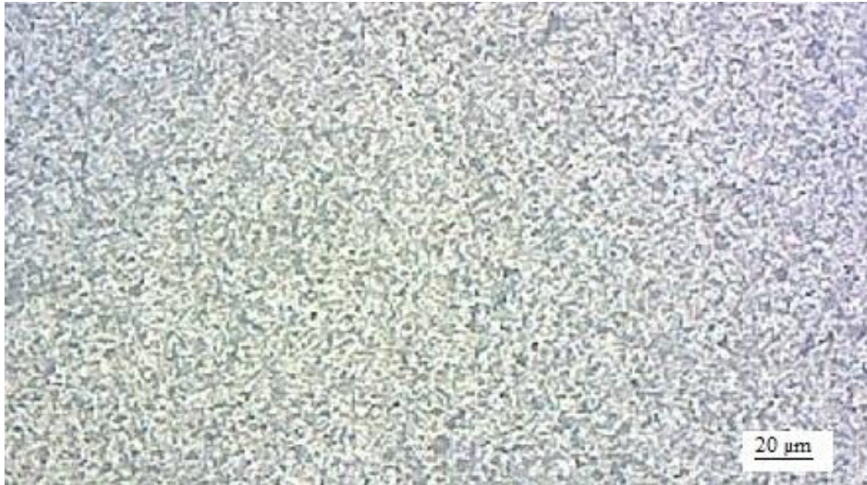
Figure No. 15 (e) Microstructure of the four pass FSPed specimen cross section
