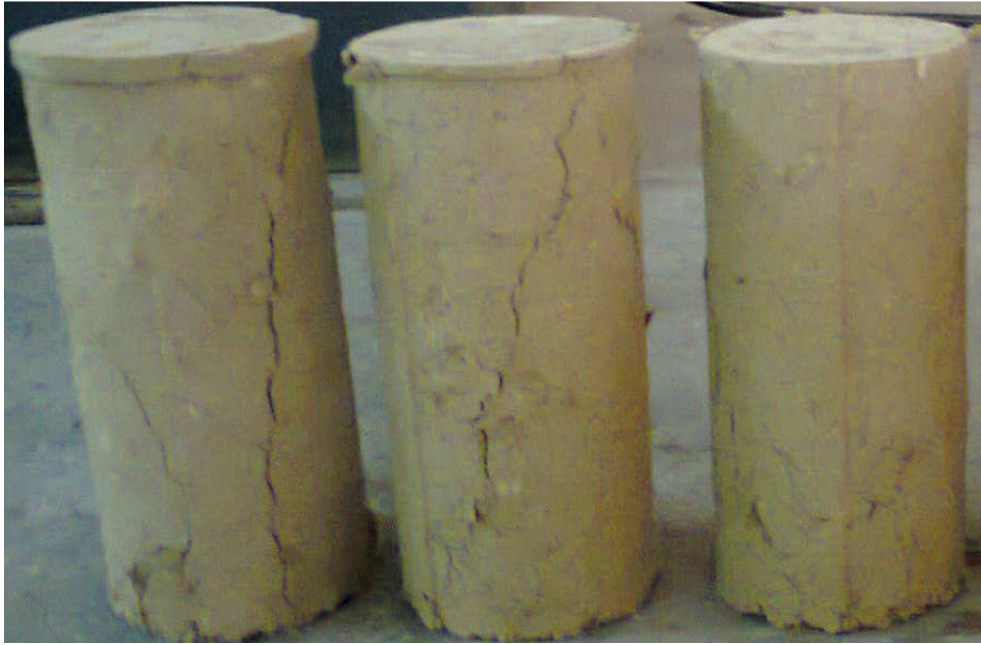
Picture 9 Failure Pattern of Sample
