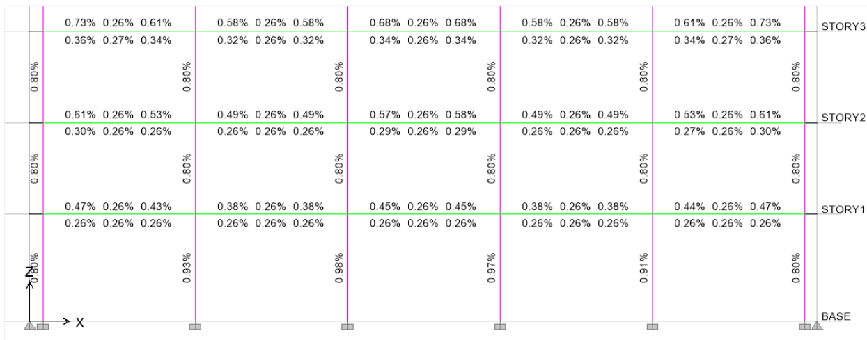
Fig 13. Rebar % in model - 2
