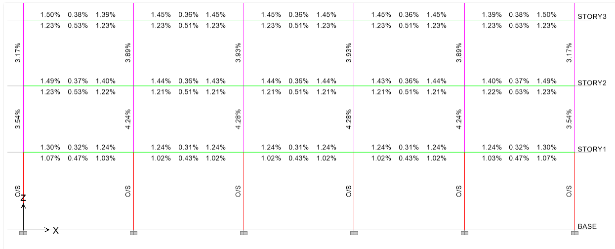
Fig 12. Rebar % in model - 1
