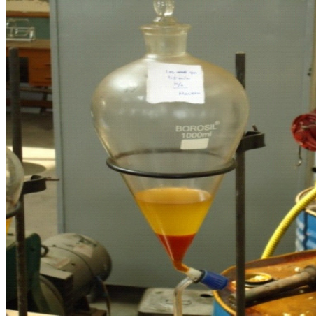
Figure 7: Alkali Catalyzed Esterification Process
