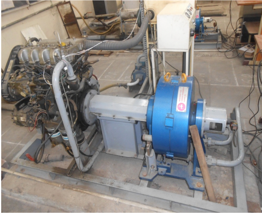
Figure 10: Actual Experimental Setup for Performance Testing (ENGINE)
