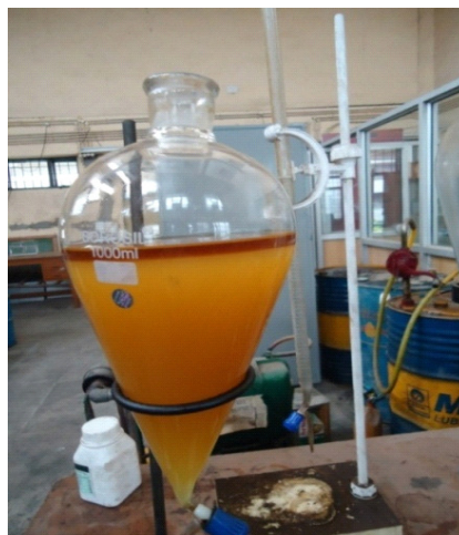
Figure 6: Acid Catalyzed Transesterification Process
