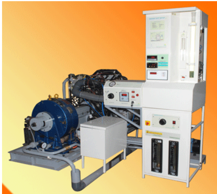
Figure 11: Actual Experimental Setup for Performance Testing (with Air and Fuel Flow Measurements)
