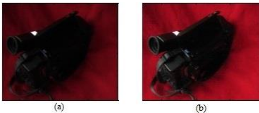
Figure 4-4 (a) original camera image with entropy = 0.42585 (b) modified image using proposed technique with entropy = 0.29843
