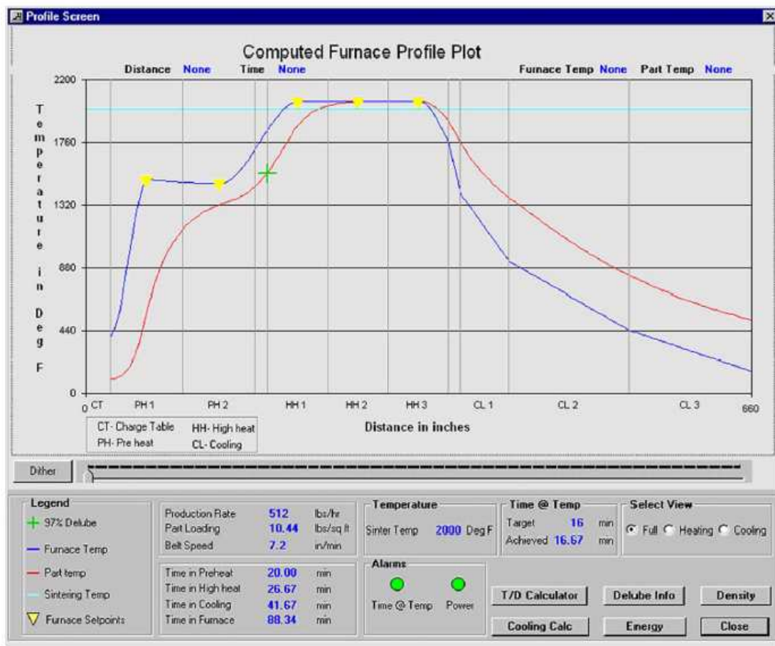
Figure 2.14 - The result illustration of FurnXpert software [10]
