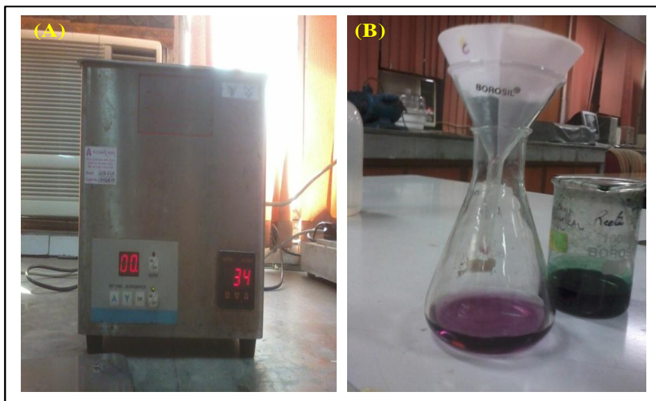
Fig.2.3: (A) Ultrasonicator instrument (B) filtering process during PANI synthesis
