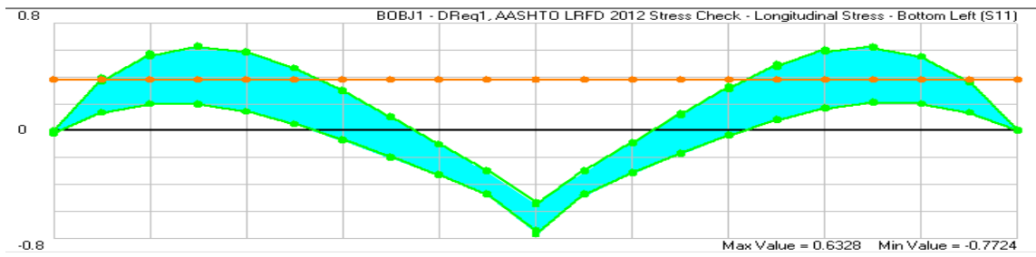
Fig 4.57 graph showing tension limit at quarter span is exceeding in 5 degree skewed non post tensioned girder.
