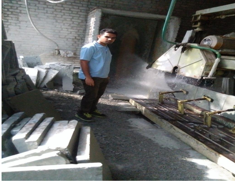
Figure 1.5: Kota Stone Cutting Operation and Generation of Slurry
