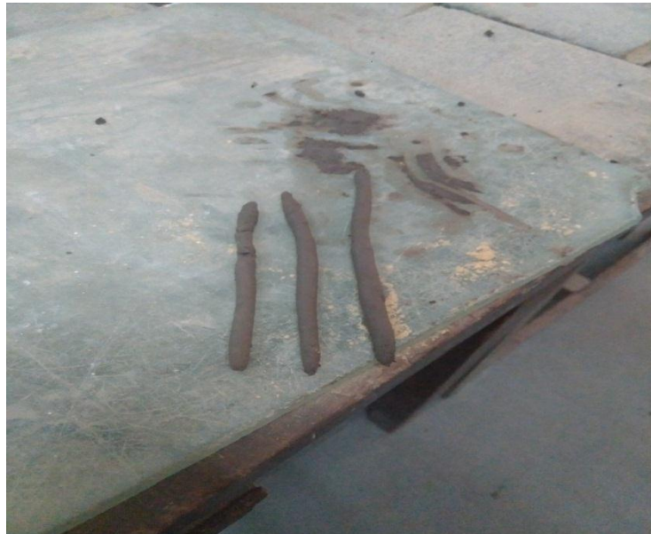
Figure 3.2: Thread Preparation during Plastic Limit Test
