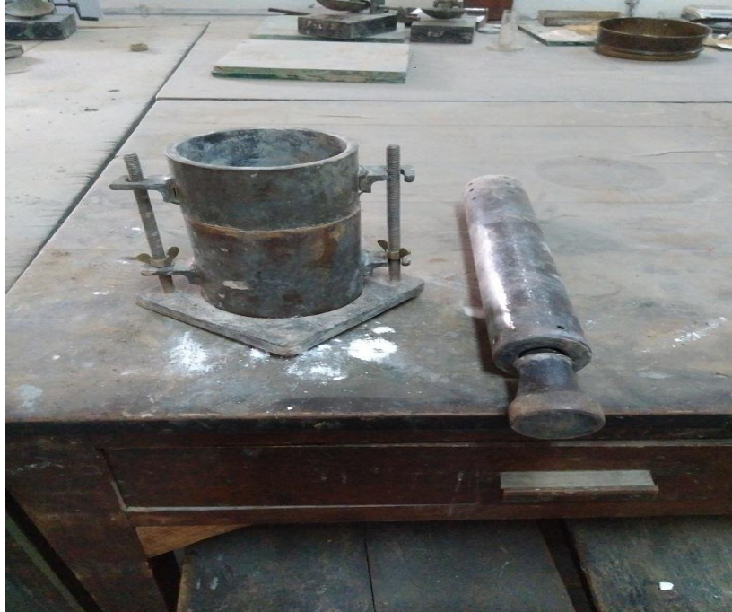
Figure 3.5: Mould and Hammer used in Standard Procter Test
