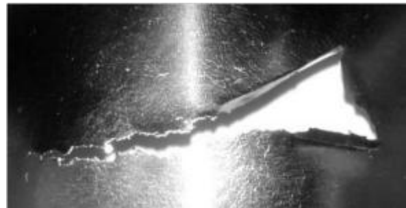
Fig 2.6: Al 0.05 mm, crack detail.
