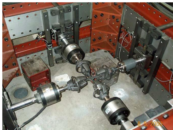
Fig 2.21: in-plane biaxial testing device
