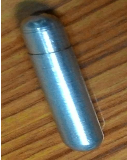
Figure 3.6: Pin prepared for wear testing.
