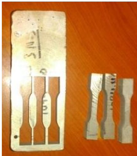
Figure 3.5: Tensile specimens obtained by Wire EDM cut.
