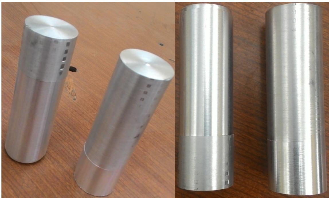
Figure 3.7: Cylindrical specimens used for turning operation.
