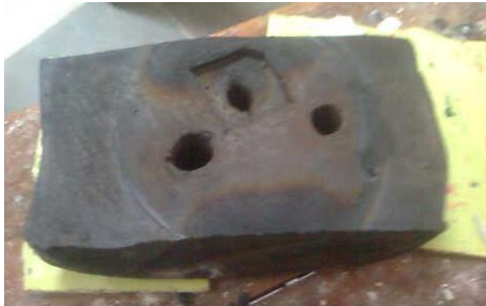
Figure 5.27 cured mould after 2 hours
