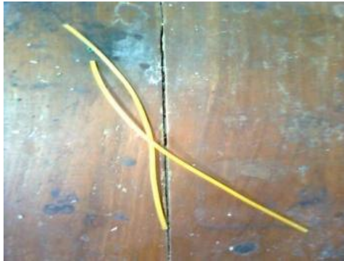
Figure 5.22 wax wires for fixing the X-ray film
