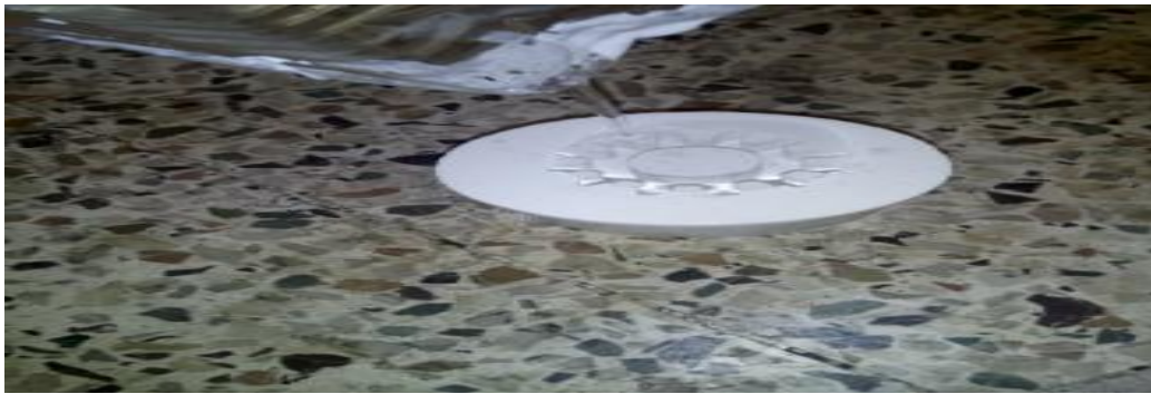
Figure 5.13 Pour the melted wax directly in the rubber pattern
