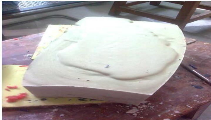
Figure 5.25 Mould after soaking for 40 min.
