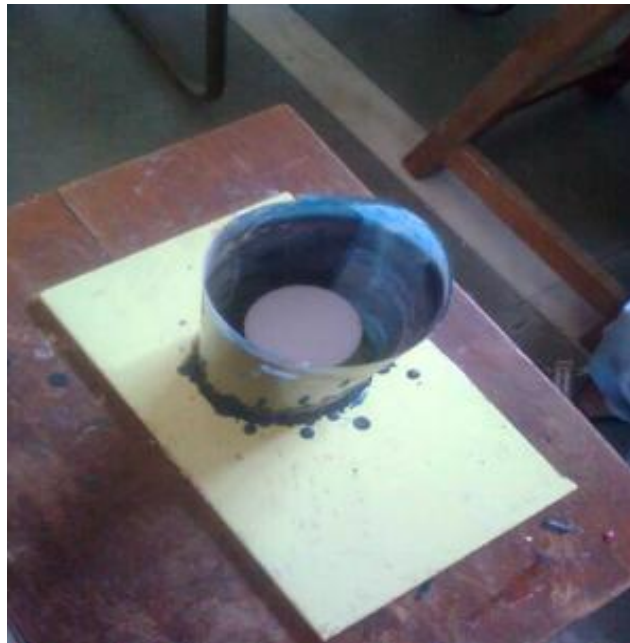
Figure 5.21 wax pattern framed in x-ray film
